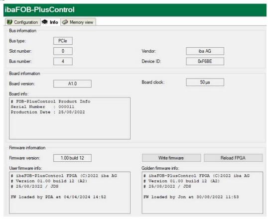
On the *Info* tab you can see information about the card and the loaded firmware. Functions for service and support, such as reloading the FPGA and updating the firmware are available on this tab.
