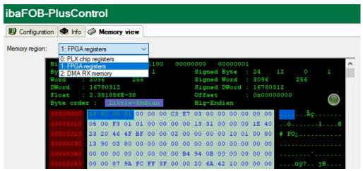
The memory view can be used for diagnostics of internal register and memory ranges.
