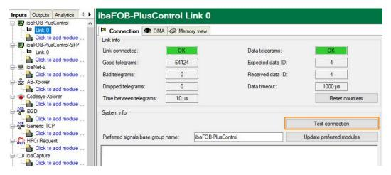
If the connection to the PLUSCONTROL system has been successfully established, the following actions are performed:
