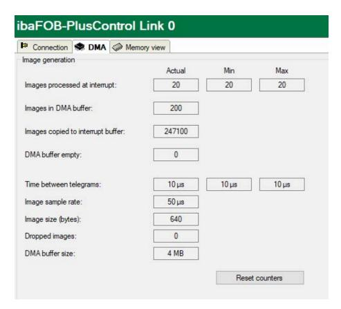
The tab gives information about the image generation (process image). An image is a dataset that the card writes into the PC system memory via DMA. This image contains all data of the measured signals within a sample on that link.
