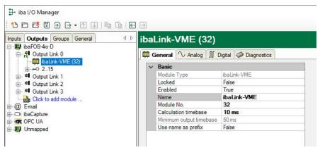
The digital signals are listed in the *Digital* tab and the analog signals are listed in the *Analog* tab. For each signal you can specify an expression using the expression builder.
