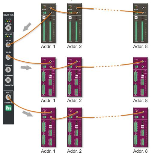
A combination of cascade mode and I/O mode at one card is possible. For example, channel 1 could connect a cascade and channel 2 could be used as output.
