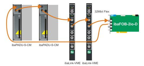
The transmission rate can be adjusted flexibly depending on the amount of data (e.g. the fastest rate is 65 bytes at 25  $\mu$ s, the maximum amount of data is 4060 bytes at 1.4 ms).
