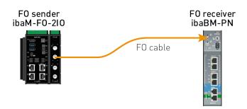
The example refers to a P2P connection with an FO cable of type  $62.5/125 \mu m$ . The light wavelength used is 850 nm.
