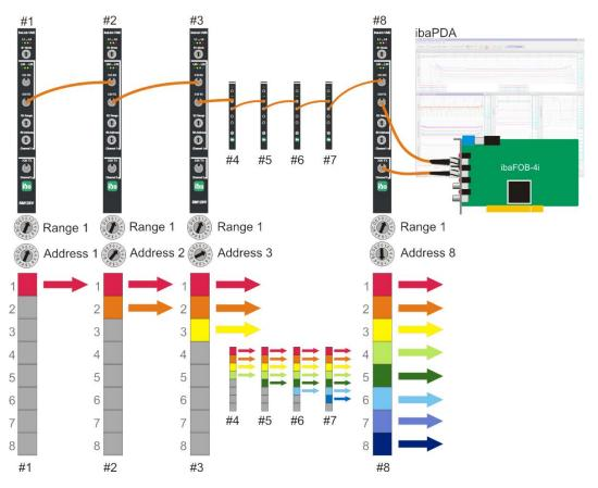
Eight ibaLink-VME interface cards are daisy-chained with each card transmitting 8 signals for the resulting daisy-chain telegram. The address switch position determines the slot to be occupied. After the last ibaLink-VME card all slots are filled with data. The FO input of the ibaFOB card receives 8 x 8 = 64 signals.
