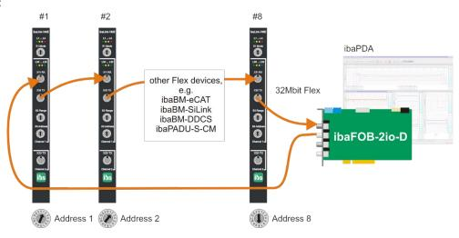
The amount of data per participant is not defined by switches like in 3Mbit mode but is allocated dynamically. According to the number of analog and digital signals configured in ibaPDA and the con-figured timebase the amount of data is calculated by *ibaPDA*.
