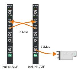
The "fast" peer-to-peer mode is also used to connect two cards, but more signals can be transmitted at a higher data rate.
