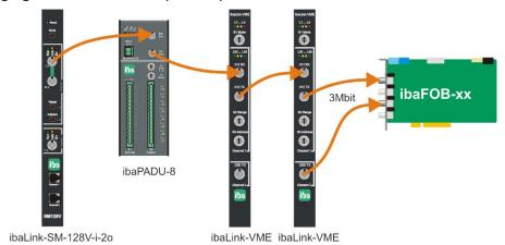
Channel 1 receives and transmits 64 analog and 64 digital input and output signals at 1 ms rate. This mode allows cascading of up to 8 devices. The S2 *Range* switch specifies the range of channels within a cascade to be transmitted over the fiber-optic link. Valid settings are 1...8 (valid for each 8 digital and 8 analog measured values). Up to 8 x (8 analog + 8 digital signals) can be transmitted in a cascade. The switch should be set to 8, when cascading is not used.
