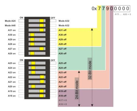
The lower four hex digits of the address have the value 0. There are no switches to change these values. The bit A16 and A17 have the fixed value 0 too.
