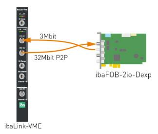
Send data to *ibaPDA* in 32Mbit P2P (e.g. installed on an HCPi system using Request mode) and receive data from *ibaPDA* in 3Mbit using the FOB Alarm output module.
