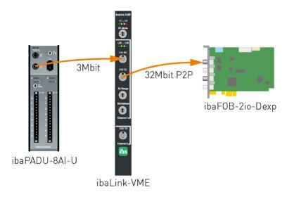
In this example, the *ibaLink-VME* is also used to send data to *ibaPDA* in 32Mbit P2P mode.
