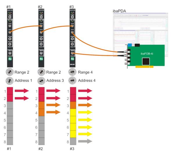
Three *ibaLink-VME* interface cards are daisy-chained, transmitting different amounts of data.
