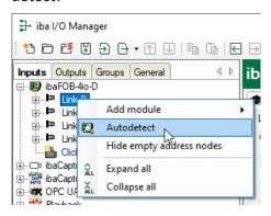
→ ibaPDA recognizes the device automatically. The device will be listed in the signal tree.
