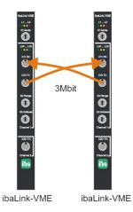
In peer-to-peer-(P2P)-mode 2 cards can be coupled to each other, exchanging data (64 analog and 64 digital signals) periodically in 1 ms (computer coupling). In this operation mode the two VMEbus memory ranges are transmitted from one card to the other. S2 *Range* switch and S3 *Address* switch are ignored. The device acts as if address switch is set to 1 and range = 8. Cascading is not possible.
