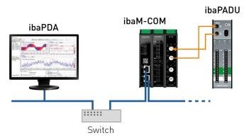
If the *ibaPDA* computer is connected to the network via a standard network adapter card, synchronous data sampling between multiple network devices at 1 ms is possible.
