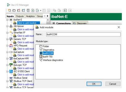
3. Once you have added the *ibaM-COM* module, to ensure a successful connection first enter the (network) address via which *ibaM-COM* can be reached.
