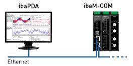
Any network topology can be used to do this. The device can either be connected to the *ibaPDA* computer directly (P2P), as shown above, or via a switch or router, as shown below. The modules connected to *ibaM-COM* are only examples.
