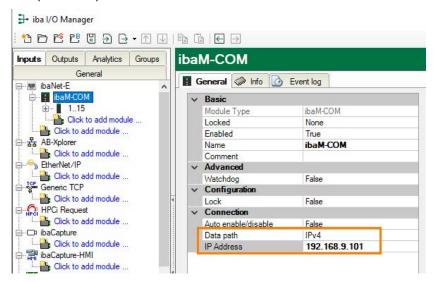
The address can either be a (fixed) IP address or the host name ("Hostname"). It is advisable to use the host name if the device is located in a DHCP network in which the network devices have not been assigned fixed IP addresses.
