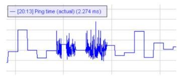
If the ping time is longer and therefore the connection quality of the Ethernet connection is not optimal, the corresponding connection is no longer highlighted in green in the connection overview, but in orange:
