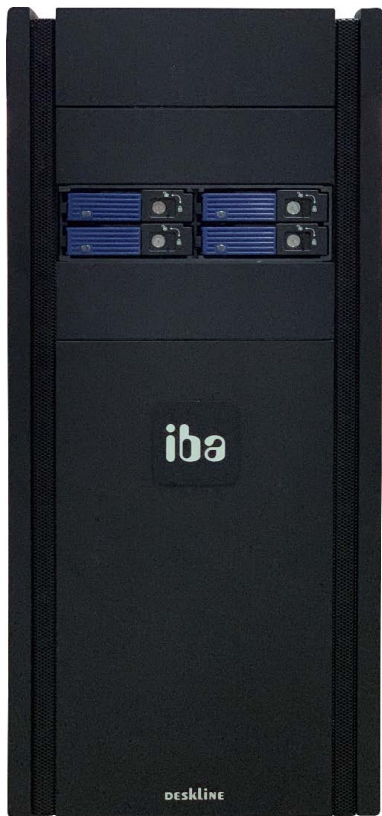
Front view with plug-in slots for hard disks
