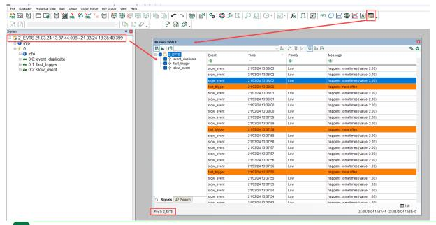
As usual, events can also be shown as text signal in ibaAnlayzer. With the new event table, it is also possible to drag an event from the table onto any trendgraph. Further, the text flags for the events contain an additional icon to indicate if it is an icoming or outgoing event.
