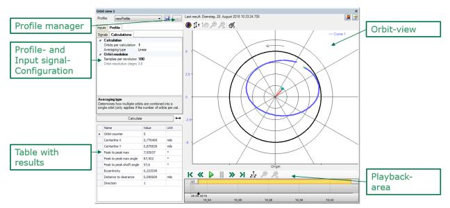
With ibalnSpectra-Orbit for instance the shaft movement inside a sleeve bearing can be monitored, analyzed and visualized. The calculated results are:
