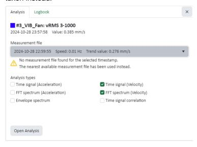
The analysis types are preselected based on the trend type. E.g. for a vRMS trend Time signal (velocity) and FFT spectrum (velocity) is selected by default. If needed, the user can change the selection before opening the analysis window.
