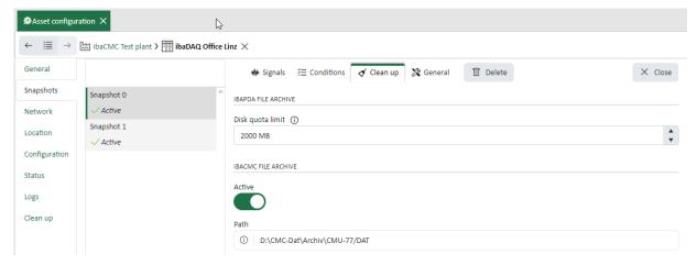
If the network connection to the ibaCMC server is lost, ibaPDA stores the files in the local snapshot folder. Once the connection is restored, the files are automatically uploaded to the server.
