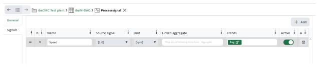
If the signal should be shown below an aggregate in the plant tree the aggregate can be linked with the process signal by drag and drop the aggregate in the *Linked aggregate* column.
