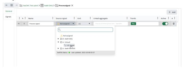
After that the unit for the process signal can be selected.
