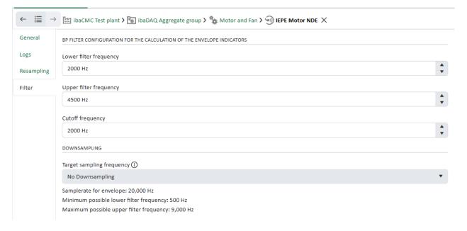
If the sensor is not connected to the CMU module, editing the filter settings is not possible.
