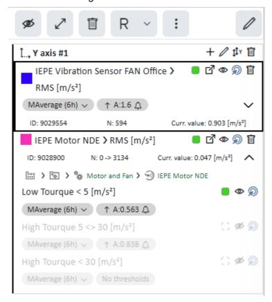
If the aggregation settings are not default which are used for the monitoring and status calculation it shows an orange dot. When hovering the dot with the mouse you get also a tooltip.
