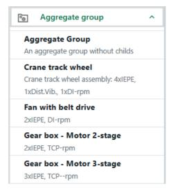
You can either use a blank template called **Aggregate Group** or one that already contains data, e.g. **Gearbox - Motor 2 stage**. In general, it is always advantageous to select the template that is as close as possible to the actual configuration to keep the amount of adjustment required to a minimum.
