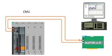
Note that the switch S1 on the CMU hardware must be set to "1" if this connection is used. Further information can be found in the CMU manual.
