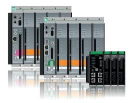
The Condition Monitoring Unit (CMU) is the measurement and analysis hardware for condition monitoring applications based on vibration measurement. Several modules can be connected to a CMU. These include modules for reading digital signals, analog signals, and vibration sensors. The TCP/IP communication protocol is used to exchange process data (e.g. shaft speed, weight, torque, etc.) with the automation environment (e.g. PLC).
