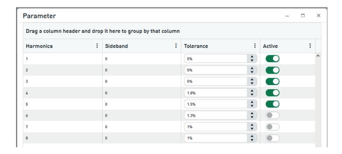
In this example the tolerance is 5 % for the fundamental and the next two harmonics. Consequently, the band width in Hz increases by rising frequencies.
