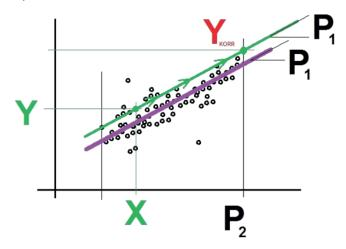
For the correlation process, the CMU starts with a new calculation of the vibration signal and the motor speed. These new values are *X* and *Y*. The CMU then makes the following calculation:
