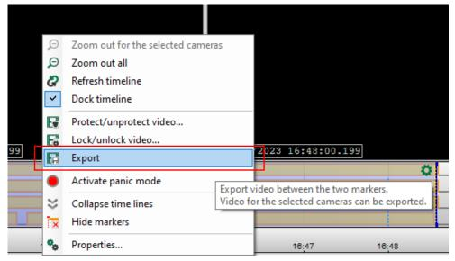
In the export grid, **Transcoding** can be enabled for each camera individually. Once enabled, the columns **Timestamp**, **Encode gaps** and **Encoding profile** are unlocked.
