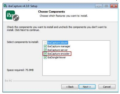
The application *ibaCapture* Encoder grabs image data from GigE cameras and provides an H.264-compliant video encoder to compress incoming video data to a video stream. This video stream can be processed and stored by *ibaCapture*.
