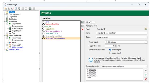
The "Time, ibaHD" allows you to configure the aggregation level time bases. By default, it is set to *Auto*. In *Auto* mode the equidistant signals are stored with time bases equal to 40 times the time base of the previous aggregation level. In *Auto* mode the non-equidistant signals have fixed aggregation levels of 200 ms, 10 s, 5 minutes, 2 hours and 1 day. You can also configure
