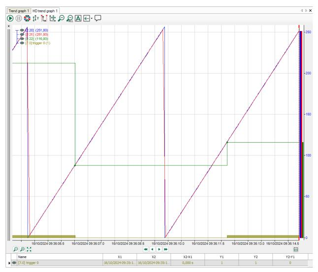
The green signal shows a non-equidistant version of the blue signal. A sample is taken each time the yellow signal changes value. The samples are shown as dots. The sample is considered constant until the next sample. That is why you see the step-wise drawing of the green signal. As long as you are on the raw level you will see the dots. When you zoom out further until the first aggregation level is used, then no more dots will be drawn.
