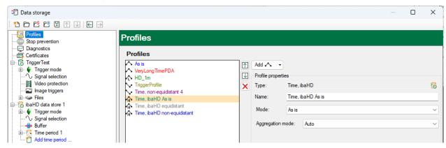
2. **Equidistant**: Signals are resampled. The new time base can be configured as an absolute time base or as a number of times the original time base. Filtering can be used
