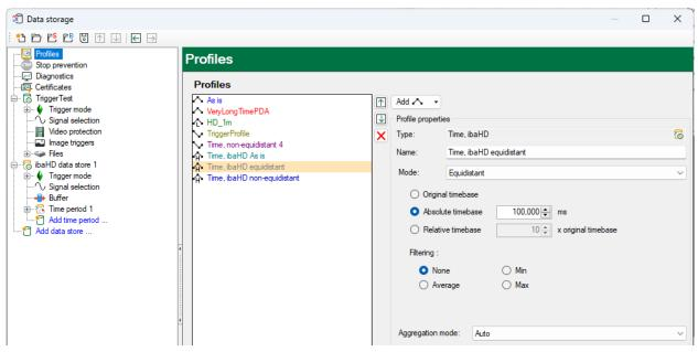
3. **Non-equidistant**: A sample is taken each time the trigger signal's value changes. So in the case of a digital trigger signal a sample will be taken on both rising and falling edges. The timestamp of the sample can be taken from the source signal or from the trigger signal. This is only relevant if the time bases of source and trigger signal are different. This profile has the same options as the standard "*Time*, *non-equidistant*" profile.
