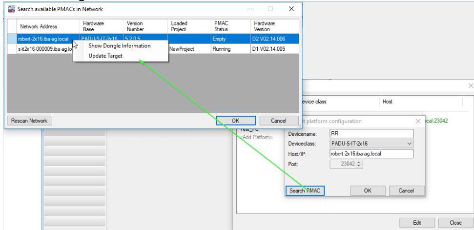
In the list of PMACs, right-click on the desired entry and start the update of the target system.
