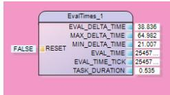
Note: The EVALTIMES module is also suitable for measuring transit times within a program. If you place two EVALTIMES blocks into the data flow, you can determine the duration of all intermediate blocks by the difference of the EVAL\_TIME outputs.
