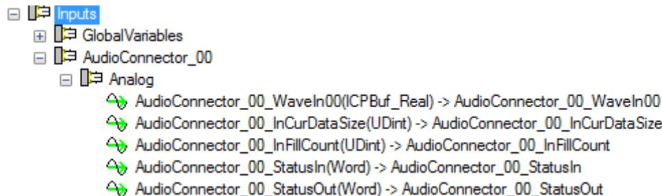
WaveIn0x: Buffered input channels (data)
