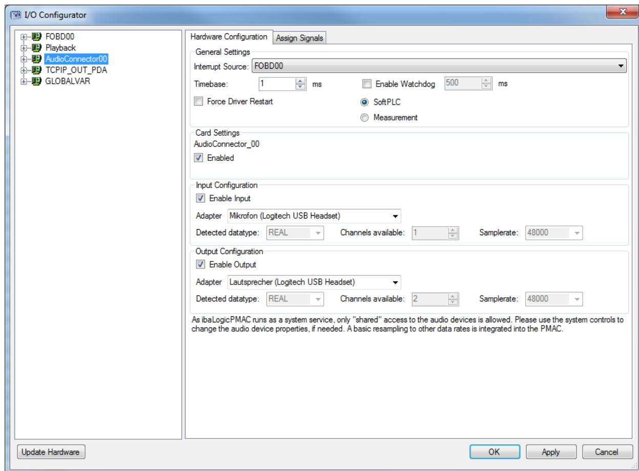
If an audio interface is detected, the AudioConnector can be found in the I/O Configurator. According to the capabilities of the interface, 1 or 2 channels are available. The sample rate can be adjusted by using the Windows system settings for the audio device.
