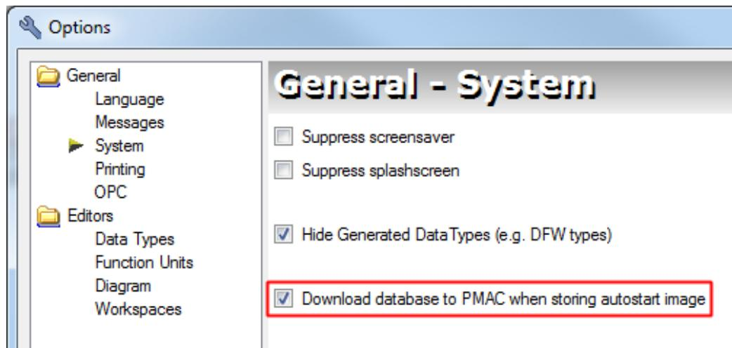
If this is active, the complete backup file is stored on the target PMAC when the function is used. ibaLogic Server can be used to upload the backup file from the PMAC.
