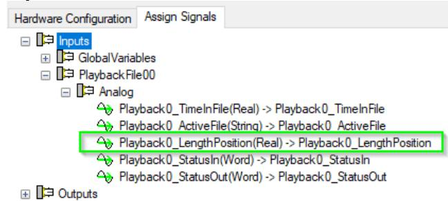
LengthPosition: Current length position when playing back length-based signals
