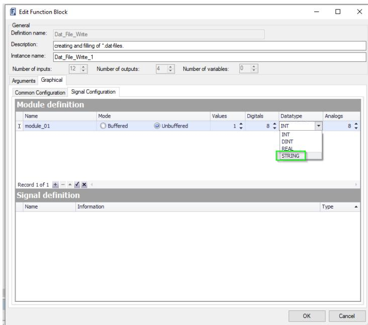
Attention: This is only possible for unbuffered values. This is not permitted for buffered signals and a corresponding message is displayed.
