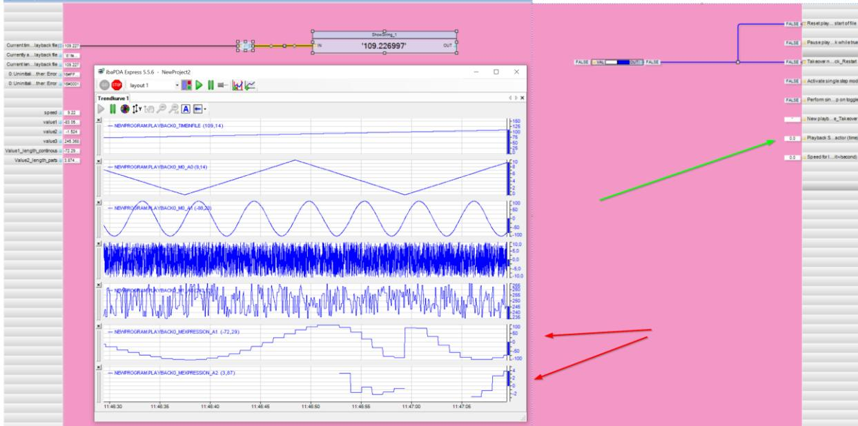
There is no speed factor set (green arrow), so the data file is played in its original speed. The internal speed factor is 1. Any other factor influences the playback speed, e.g. 2 = 2 times the speed, 0.5 = half the speed, etc.
