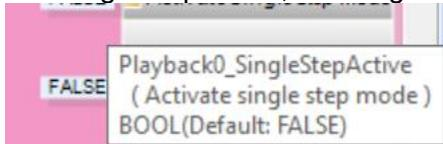
In this case, a value change at the DoStep output causes the playback to advance by the timebase of the IO-configuration. To jump directly to the next sample, the output speed factor must be configured accordingly.
