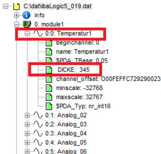
The modulname can be renamed by "Module\_Name\_0: MeinModulName;" But here all module names which should be renamed must be written here in a single row. The names **Module\_Name\_x** are fixed! Attention: Only 1024 Bytes are available for the rename. Because of the 14 chars of the standard name you are limited in your dynamic module names.
