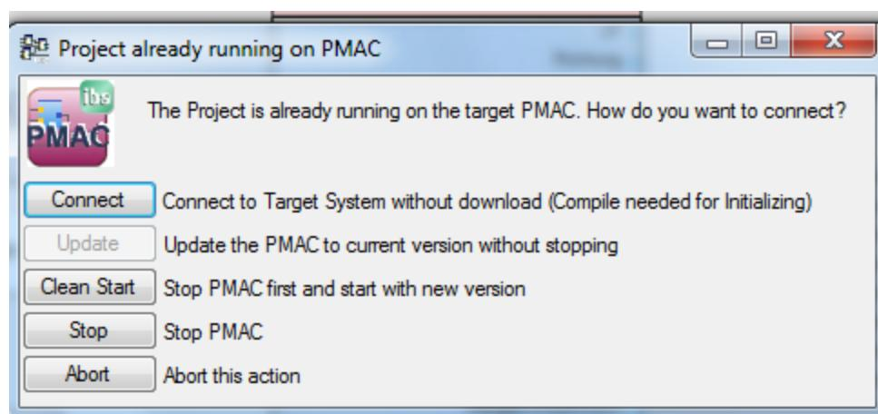
If the hardware configuration and the active project are identical with the version running on the target PMAC, he can CONNECT without stopping the system. As additional choices he can perform a CLEAN START with a Stop/Start in the background or just STOP the running PMAC.
