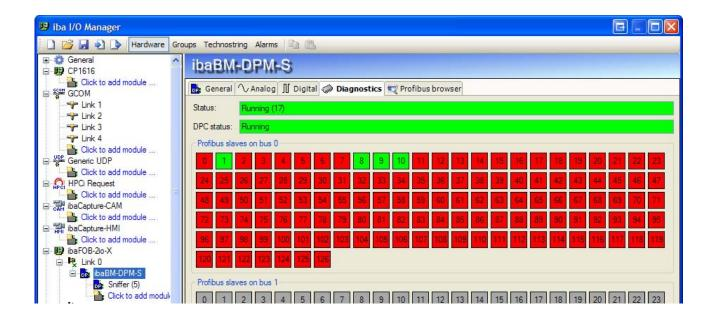
In the old mode a slave can have only 2 states: slave is ok or not ok. A slave is ok if it is on the bus and the master is accessing it. The new diagnose gives more information.
