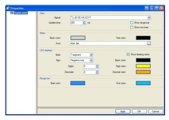
In the properties form you can setup how many digits are displayed. You can also specify how many of these digits are used as decimals. If the signal value is larger than can be displayed by the number of digits then the meter displays E for all its digits. This means overflow. If the signal is no longer valid then the meter displays – for all its digits.
