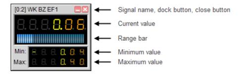
In v6.20.0 the digital meters from pda version 5 are back. A digital meter shows the actual value of an analog signal. Optionally it can show the minimum and maximum value of the signal. It can also show a range bar that shows the position of the current value between the minimum and maximum value of the signal. The digital meters can be floating or they can be docked in the digital meters panel. The digital meters panel can be shown via the View menu.
