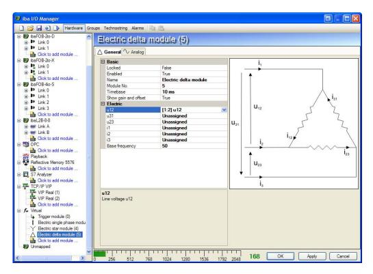
On the general tab you have to specify the input voltages and currents. You also have to specify the base frequency in Hz. The timebase of the module can be set to 1/base frequency because a new value will be available only every period.
