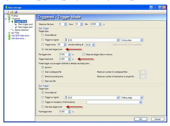
The trigger mode form also contains a new property called "Trigger dead time". This property works on every start trigger type (signal trigger, periodic trigger and start trigger pool). The trigger dead time determines the time after a trigger occurs that subsequent trigger occurances are ignored. So if the dead time is set to 5 seconds then in the 5 seconds after the first trigger happens all other triggers are ignored.
