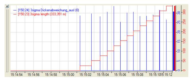
The signal bars always show the current value of the signals no matter if the length is constant or if it is changing. In previous version the signal bars only changed when the length changed.
