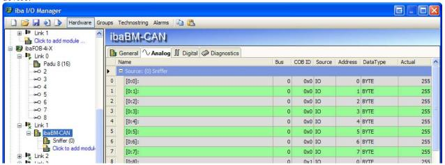
The analog and digital tabs show the current configuration. You can also see the actual values of the signals here.
