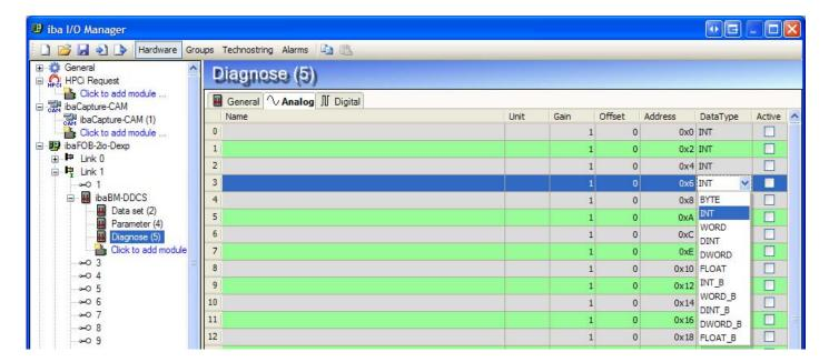
There is also a third module type called diagnose module. This module can be used to measure data from the internal memory of the DDCS device. Currently it is only used for troubleshooting by iba support.
