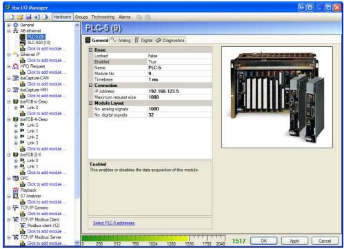
The SLC-500 module in pda is very similar to the PLC-5 module. The only difference is that the addresses of the SLC-500 have other limits than the addresses of the PLC-5. The file number is limited to 255 and the element number is also limited to 255.
