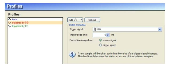
The normal profile and the QDR profile already existed in pda versions prior to 6.27.0. The non-equidistant profile is new. This profile will take a sample each time the value of a trigger signal changes. The trigger dead time determines the minimum amount of time between samples.
