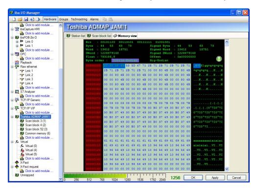
There are 2 types of modules you can add to the Toshiba ADMAP JAMI1 interface: scan block module and common memory module.
