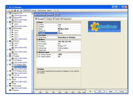
On the general tab of a Modbus client module you first have to enter the IP address of the Modbus server. You can set the port number. By default it is set to the standard Modbus port 502.
