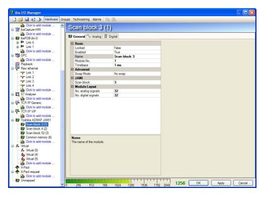
The common memory module is able to measure the 128kB of common memory. On the general tab you can specify the swap mode and the number of signals.
