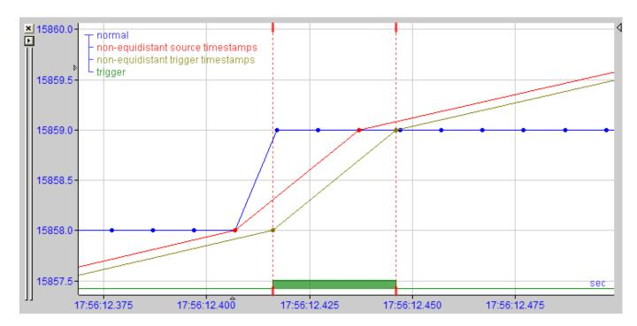
When the trigger signal and the source signal have different timebases then you can choose which timestamps to use for the non-equidistant signal. The screenshots shows the two options. The blue signal is the source signal. The green digital signal is the trigger signal. The source signal is sampled at 10ms. The trigger signal is sampled at 1ms. You see that the trigger value changes at a time that doesn't correspond with a sample of the source signal.
