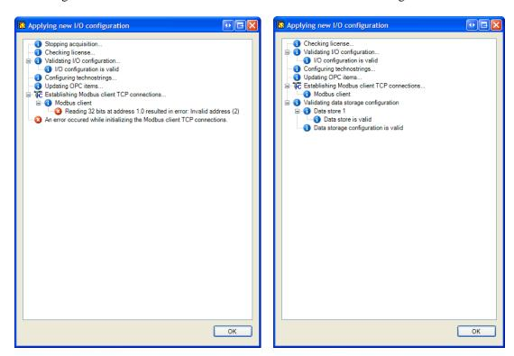
At the start of the acquisition pda tries to connect to the Modbus servers and it tries to read the data once. If the server returns an error then it is shown in the validation form.
