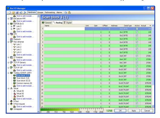
For a digital signal you have to specify the address and the bit number. The bit number goes from 0 to 31.
