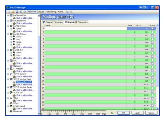
For each analog signal you have to specify the slave number and bit number. The bit number corresponds with the coil number or discrete input number. The valid range is from 0 to 65535. Like the analog register number you can switch between decimal and hexadecimal notation via the context menu.
