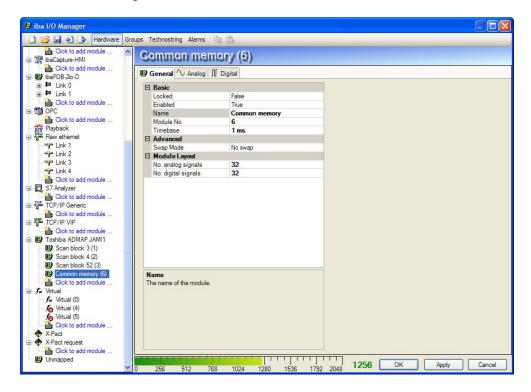
The analog and digital signals are configured in the same way for both module types. For an analog signal you have to specify the address (in hex or decimal) and the datatype. The actual column shows the current value of the signal. By clicking on the "actual column" header you can switch between raw and scaled view of the value. By clicking on the "address column" header you can let pda calculate the addresses based on the datatype of the signals.
