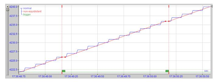
The screenshot shows the result in ibaAnalyzer. The blue signal is the original signal measured with the As is profile. A copy of the original signal is measured with a non-equidistant profile. This is the red signal. The trigger signal was the green digital signal. You see that each time the trigger signal changes a sample for the red non-equidistant signal is generated.
