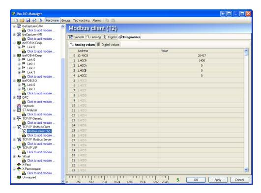
The last tab is the diagnostics tab. This tab shows the current values of the measured signals.
