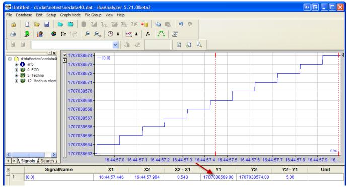
The same applies for analog signals with 64 bit floating point data type (DOUBLE). The double data type is preserved in the dat file and ibaAnalyzer will display and calculate the data correctly.
