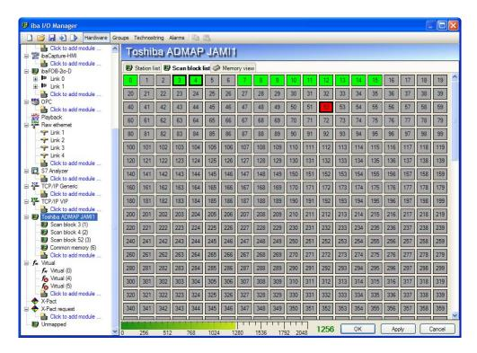
The second tab shows the scan blocks. There are 1024 boxes and each box corresponds to a scan block. A scan block is healthy when there is a talker for that block, so when there is a station writing to that block. The healthy blocks are shown in green. The unhealthy blocks are shown in red when pda is measuring from them and in gray otherwise. The blocks that pda is measuring have a thick border.
