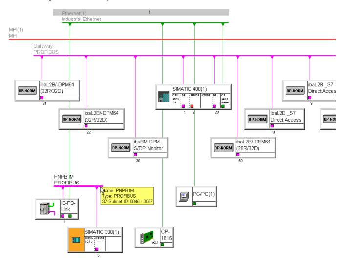
The PG is connected to the industrial Ethernet network. The IE/PB link has IP address 192.168.123.207. The target CPU IM151-7 is connected to the profibus PNPB IM and has profibus address 5. The profibus network itself has a subnet ID 0045-0057.
