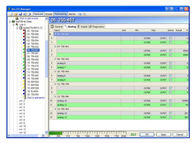
The analog tab shows the analog input signals grouped by terminal. When you click on a signal row then the corresponding terminal node will be selected in the tree. When you select a terminal in the tree then the corresponding signal row will be selected.
