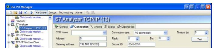
S7 routing works also in case you need to make more than 1 network transition to reach the target. In S7 analyzer you always have to specify the gateway address of the first gateway and the subnet ID of the network the target is connected to. The route in between is automatically determined by the PLCs and CPs in the path.
