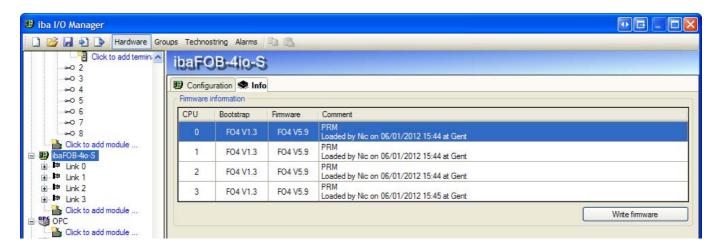
Pda can now update the firmware on FOB, FOB-S, FOB-X, FOB-TDC, FOB-SD and L2B boards. This functionality is copied from ibaDiag. The interface nodes for these boards have a new tab 'Info' that shows the loaded firmware version on the different CPUs. There is also a button to write the firmware. This opens the same firmware loader dialog as for FOB-D.
