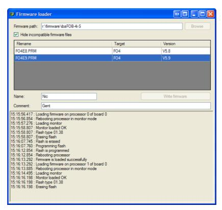
When you press write firmware the selected firmware file (.PRM file) is written to all CPUs on the board.
