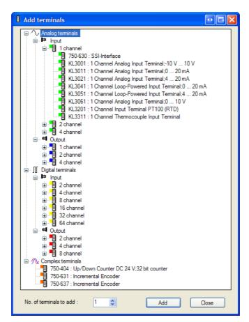
The terminals are sorted by type (analog, digital, complex), by direction (input, output) and by number of channels. The color of the terminal icon corresponds with the color of the actual terminal.
