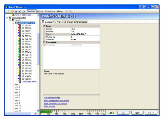
The ibaNet750-BM-D device is the successor to the ibaNet750 device. It supports most Wago and Beckhoff terminals. The new device has 2 modes determined by the mode switch S1:
