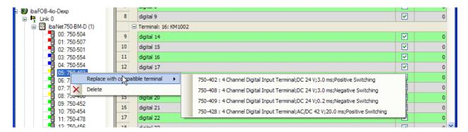
The autodetect procedure can detect the type number for the analog and complex terminals. So for the analog and complex terminals there is no need for a replace function.
