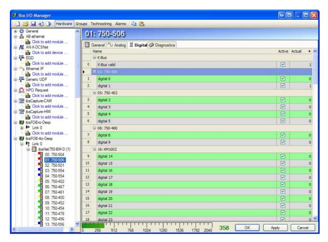
The digital grid contains 1 virtual terminal called the K-Bus. The K-Bus is the name for the internal bus between the ibaNet750-BM-D device and the terminals. This virtual terminal contains 1 digital input signal called K-Bus valid. It will be 1 when the K-Bus is ok. It will be 0 when the K-Bus is not ok (e.g. not properly terminated). When the K-Bus is not ok then all the signal values will be 0 as well.
