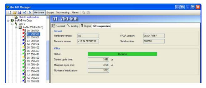
The last tab is the diagnostics tab. It shows some general version information about the device. It also shows the status of the K-Bus. The status can have the following values:
