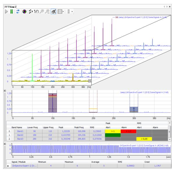
In ibaPda < V6.30.0 the FFT View contained one graph. This graph corresponds to the graph visible at the top of the screenshot. We will refer to it as the <u>main window</u>. In this new version, four sub windows have been added. They can be switch on or off independently by using the toolbar:
