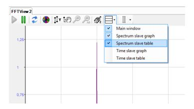
By using the toolbar one can enable the spectrum slave graph and/or the spectrum slave table. An example screenshot is shown here:
