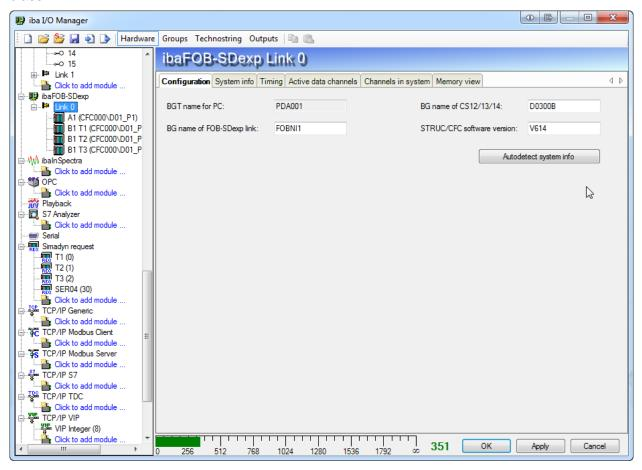
The interface link shows different tabs similar to the old boards. On the configuration tab you can define the name of this board. The name and software version of the rack this link is connected to can be automatically filled in by clicking the "Autodetect system info" button.
