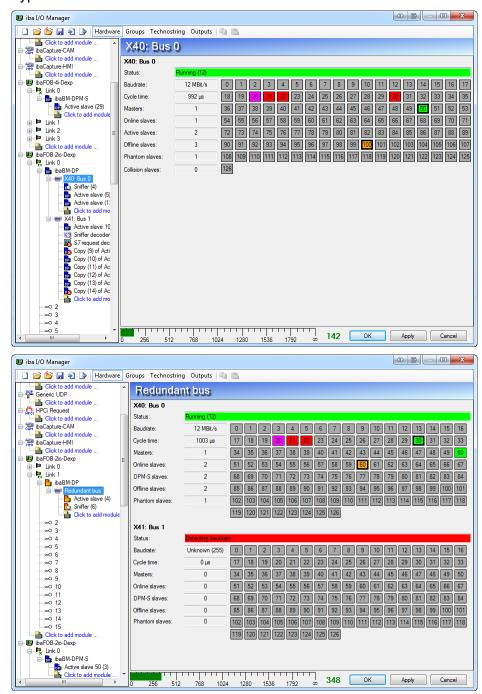
The bus node shows diagnostics for the single profibus or for both profibuses when redundancy mode is enabled. You can click on a slave to go to the profibus browser.
