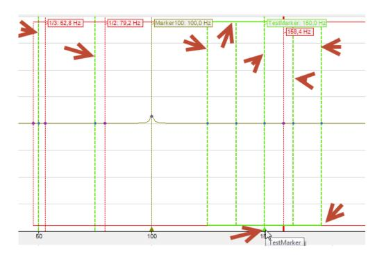
If you press the DEL button while a marker is hovered, it will become invisible. You can reenable this marker by changing its visibility state in the properties dialog of the FFT view.
