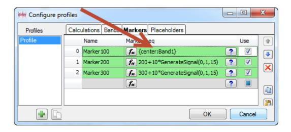
Vice-versa, one can use the center frequency of a marker in the definition of a band.
