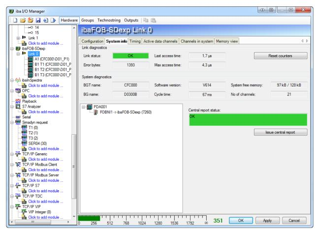
The system info tab shows diagnostic information about the link and about the connected system. You can press the "Issue central report" button to register the FOB board in the system. This is only required for debug purposes. Normally ibaPDA will automatically register the board when needed.
