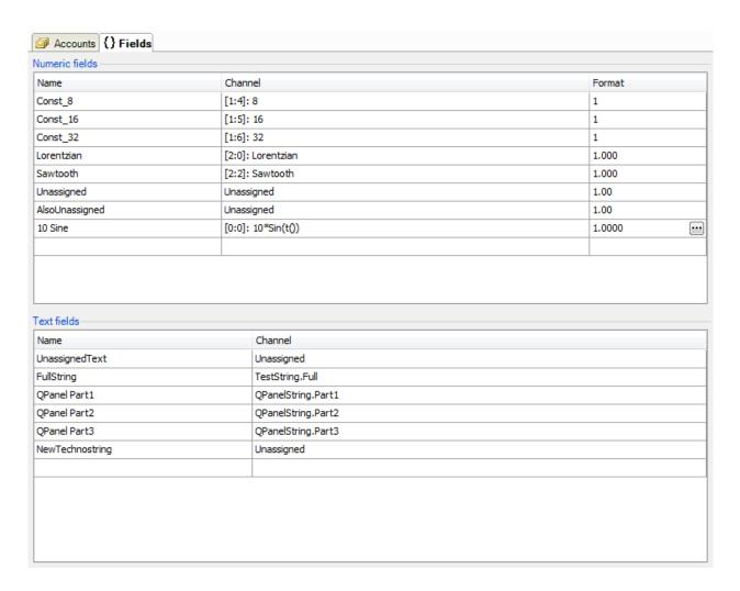
In the Fields tab, placeholders can be defined that can be used in the e-mail messages, similar to how HD events can be configured. Numeric fields can represent the value of standard analog and digital signals while text fields correspond to Technostrings. Field names cannot
