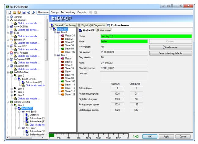
On the profibus browser there have also been some changes. You can now see the name of the device and the available licenses (e.g. redundancy mode). You can also see how many active slaves and signals there are configured and how many there are maximally allowed.
