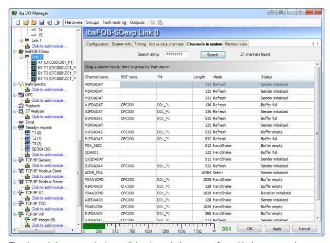
The channels in system tab shows all the channels that are configured in the connected system. These are not alone the configured data channels of the board but also all command and acknowledge channels and also all other channels that have nothing to do with ibaPDA.
