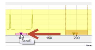
By pressing and holding the SPACE bar the system will also select the corresponding band in the band table (even if the band table is not visualized).
