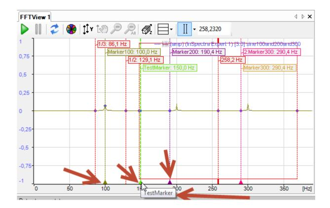
If you hover over such triangle, a tooltip containing the marker's name will appear. In case the marker is a linked InSpectra Expert marker, also its module name and number will appear in the tooltip.
