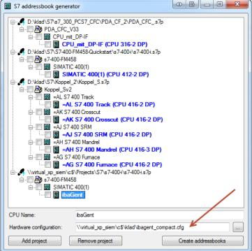
In the ibaPDA S7 addressbook generator you can now add the path of the exported hardware configuration file on the rack or CPU node. If you do this then the generated addressbook will contain the symbols for the different profibus slaves. On the sniffer module there is a "Browse profibus symbols" hyper link. Click this to open the symbolic profibus browser.
