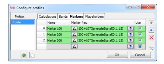
It is possible to use a placeholder of a band in the definition of a marker. This way, the center frequency of a marker can refer to the center of a band.
