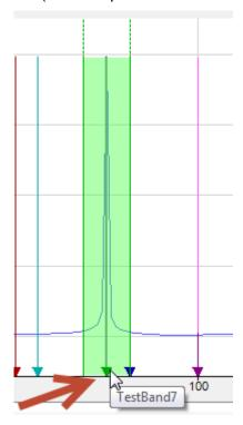
In case many bands are defined and set to visible, with the use of line bands, it is easier to interpret the bands, the labels and the curve than with the use of wide bands:
