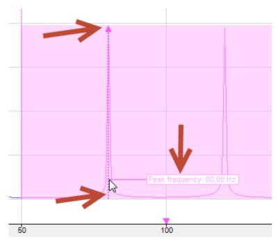
Note: this peak frequency line segment is only visible if the peak frequency signal of the corresponding InSpectra Expert band is active.
