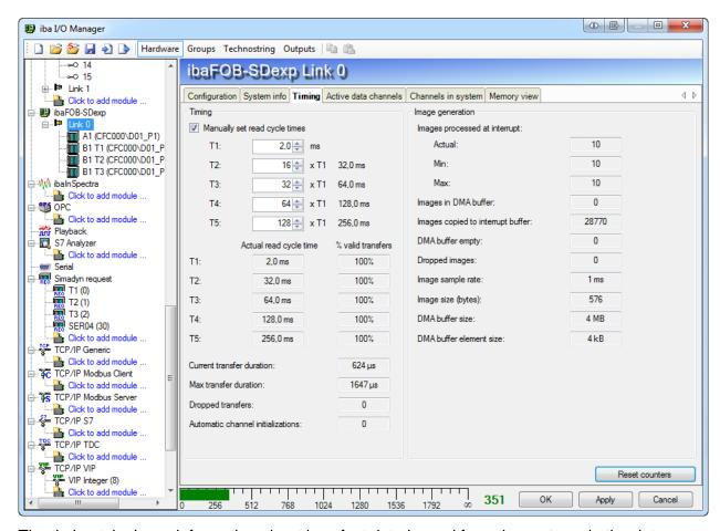
The timing tab shows information about how fast data is read from the system via the data channels on the left side. It shows information about how fast the data is transferred via DMA into the main memory of the PC on the right side.
