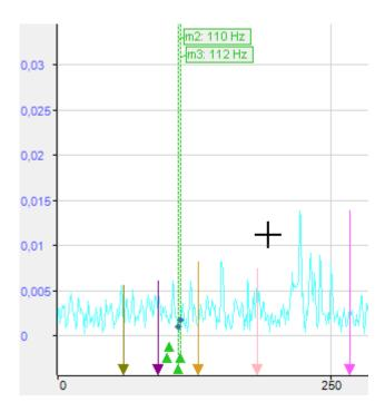
The four green upward triangles are markers. The two left markers are collapsed. The other triangles pointing downwards are bands (shown as line bands).
