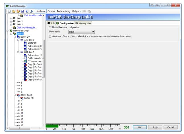
In ibaPDA you configure the flex mirror mode of a FOB-D link on the configuration tab of the link. There are 3 possible modes:
