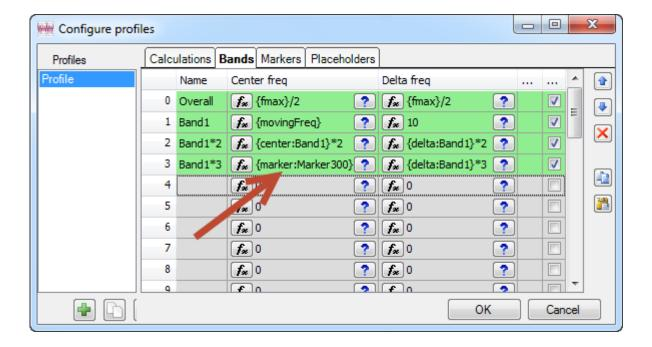
One can also use the marker or band placeholders in the definition of the limit, time or deadband of a band event. Note that markers do not support events.
