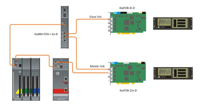
3. Connect the TX of the last flex device to the RX of an ibaBM-DIS-i-8o-D device. Connect one output of the ibaBM-DIS-i-8o-D to the ibaFOB-D in the master ibaPDA system and one output to the ibaFOB-D in the slave ibaPDA system.
