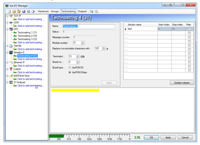
One technostring per board can be measured. The only thing that has changed with previous versions is that you now can set the board type to choose between the SD/TDC or SDexp/TDCexp boards.
