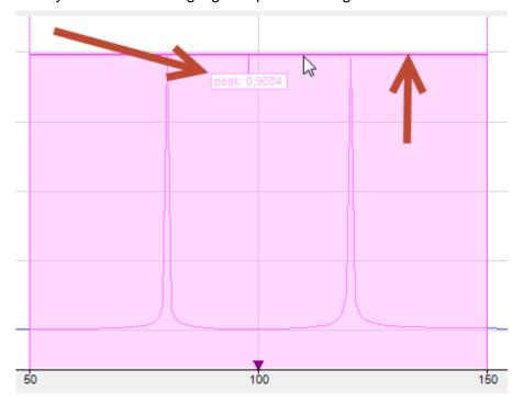
Note: this peak line segment is only visible if the peak signal of the corresponding InSpectra Expert band is active.
