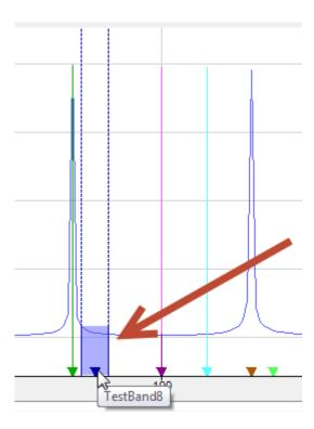
• In case the line band is not collapsed, the wide band will have the normal height (which depends on the other band settings):
