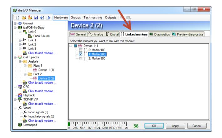
In this TAB there is a tree containing an overview of all other InSpectra Expert modules and their markers. Checkboxes are used to indicate which markers are linked with the selected module.
