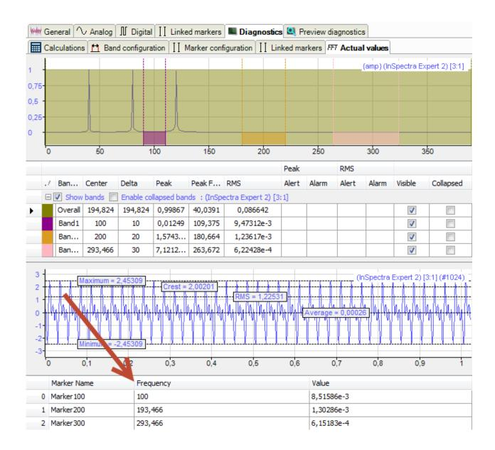
The visualization settings of the bands and markers are loaded from the registry. However, in the spectrum chart of the I/O manager all labels are disabled. You can only access the labels by pressing and holding CTRL.
