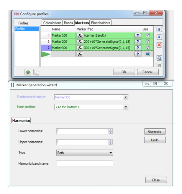
The values of the markers markers can be monitored in the diagnostics and the preview diagnostics TAB. You can read a marker's current frequency and the corresponding value of the spectrum in the table at the bottom.
