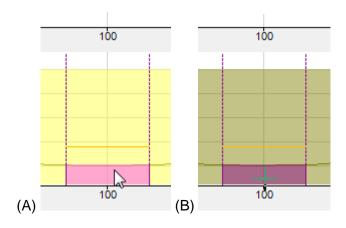
5) Enable collapsed bands: The functionality of collapsing bands is similar to the functionality of collapsing markers. In case the setting enable collapsed bands is on, a triangle appears at the center of the band. The triangle of a collapsed band is an upside down version of the triangle of a collapsed marker. This difference allows distinguishing easily between collapsed markers and bands.
