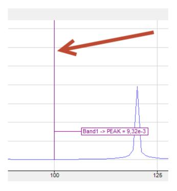
One can still visualize a wide version of a hovered line band by pressing and holding the SPACE bar:
