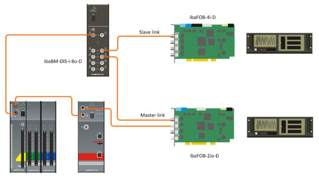
The advantage of modes 2 and 3 is that the slave link can still measure the data when the master PC has been shut down. The advantage of mode 1 is that you can mirror up to 4 different flex links with a single ibaFOB-4o-D.
