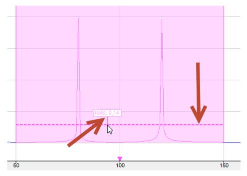
Note: this RMS line segment is only visible if the RMS signal of the corresponding InSpectra Expert band is active.
