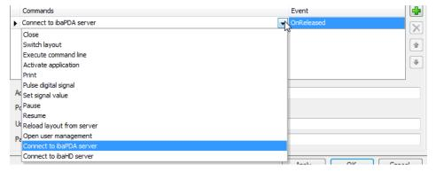
The QPanel button control also has some new commands related to user management. First there is a command to open the user management form. There is a command to reload the layout from the server. This requires the current logged in user to have the *Load layout from*
