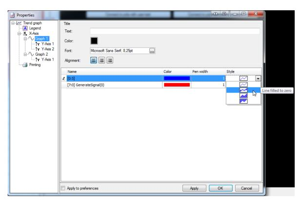
There are also new paint styles for the analog signals. Before 6.35.0 there was only line and filled. In 6.35.0 there are now 3 filled styles:
