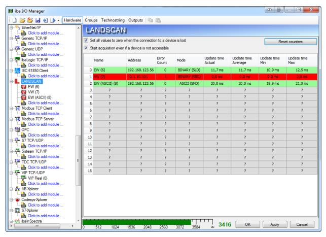
The LANDSCAN interface shows a connection grid. There is one row per connection to a scanner. Each LANDSCAN license allows 2 scanners. A maximum of 16 scanners is supported.
