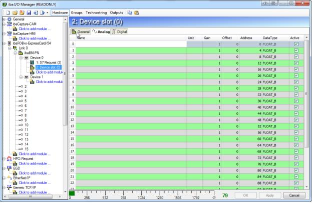
The device slot module allows you to configure the data bytes of the slot. You can configure the number of analog and digital signals that are mapped to that slot. For the analog signals you have to configure the byte offset within the slot and the data type. For the digital signals you have to configure the byte offset within the slot and the bit number (0...7) within the byte.
