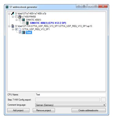
The TCP/IP TIA mode requires an addressbook to be able to read data from a CPU. The S7 operand column is not shown in the analog and digital signal grids in this mode. The addressbook generator can now open TIA Portal projects. It supports TIA portal v13 projects. An S7 addressbook contains comments in one language and a TIA project can contain comments in multiple languages. So in the addressbook generator you can select the language you want in the addressbook.
