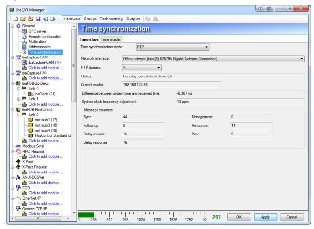
The time synchronization configuration has been moved from a tab on the general node to a separate time synchronization subnode of the general node. On the time slave tab you can configure the time synchronization mode used to synchronize the system clock.
