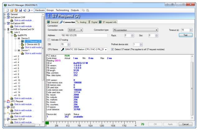
The request modules have a connection tab where you can determine how ibaPDA communicates with the management FB. The connection settings are the same as the ones of an S7-Xplorer module. There are only 2 additional settings:
