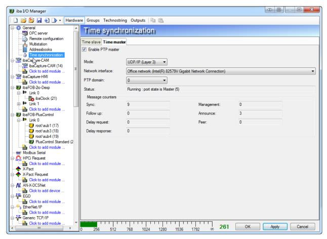
The time master tab allows you to enable PTP master. You can even enable this when the PC is synchronized by another time synchronization mode. E.g. this PC can be synchronized by DCF-77 and it can synchronize other ibaPDA systems via PTP.
