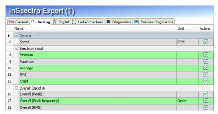
The (direct) speed was added to the analog signals of the Expert module. In this way, the speed can be recorded in a data store.
