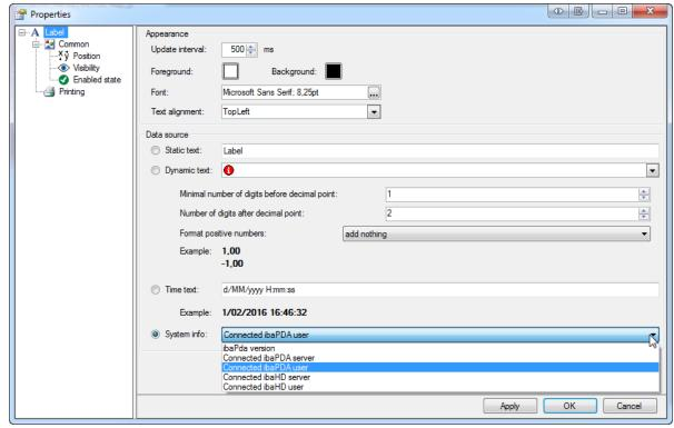
The QPanel label control has also been updated with extra system information. It can now show the connected ibaPDA server and user. It can also show the connected ibaHD server and user.
