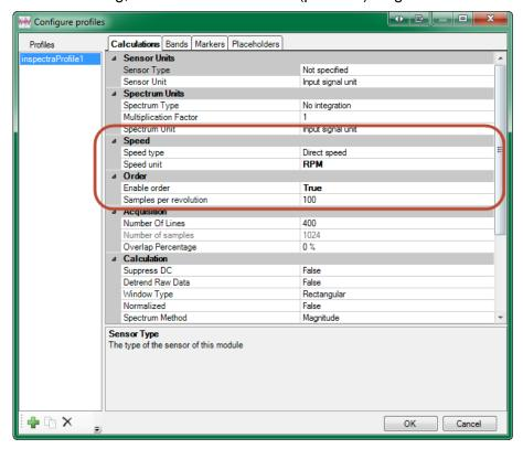
Several speed units are supported. The system can parse the unit of the speed signal automatically.
