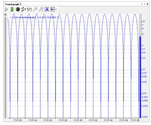
The trend graph now supports a logarithmic Y scale. To enable it go to the Y axis properties and set the scale type.
