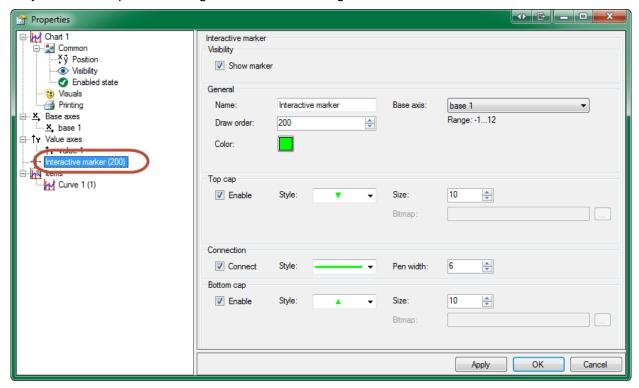
The interactive marker can be customized in the properties dialog of the ibaChart. It can be enabled or disabled via the toolbar. When enabled, a table appears at the bottom of the view. This table contains the x and y values of all curves defined at the selected tick position.
