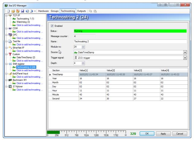
The shift register technostring works in the same way as the shift register module. The difference is that the input is now a technostring instead of a signal. For each section "s" of the source technostring new sections "s[1]", "s[2]", ... "s[n]" (n = depth of shift register) are created in the shift register technostring. The values are shown in a table in the I/O manager. The table has a row per section of the source technostring and a column per position in the shift register.
