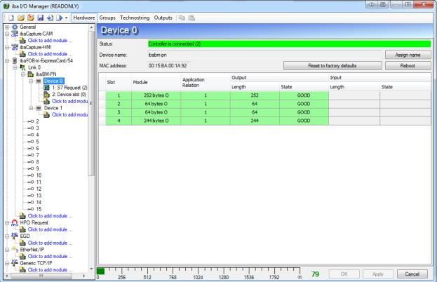
In the I/O manager the ibaBM-PN module has 2 sub nodes, one for each active device. The device node shows the current status of the device, its PROFINET device name, its MAC address and the slot configuration.
