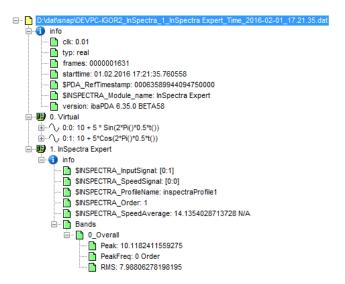
Normal dat files include 2 new module info fields for Expert modules: profile name + order enabled.
