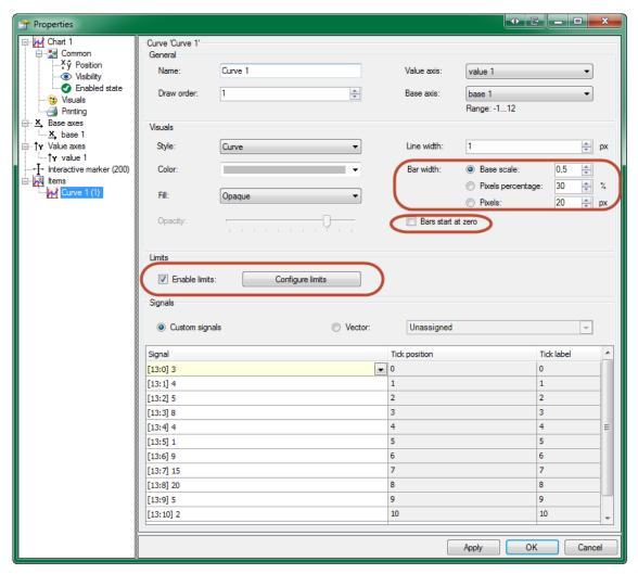
The curve style "Lines" was removed. Instead, the user can use the curve style "Bars". The new setting "Bars start at zero" determines whether the bars start at the bottom of the graph or at zero.
