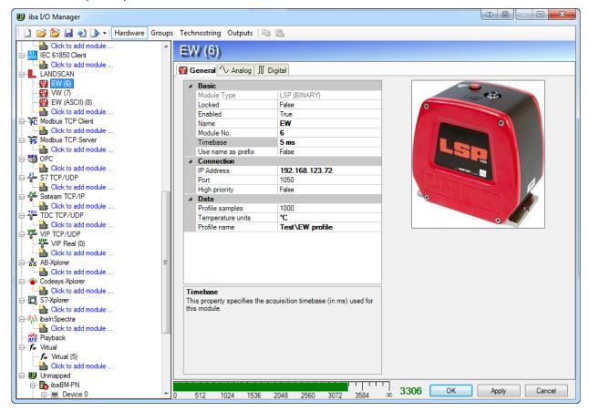
You have to enter the IP address of the scanner and the port number. You can configure the temperature unit (°C or °F). The scanner always sends 1000 samples per line in binary mode. You can reduce the number of samples via the *Profile samples* property. If you set the *Profile samples* to 200 then ibaPDA will take every 5<sup>th</sup> sample. There is no aggregation done.
