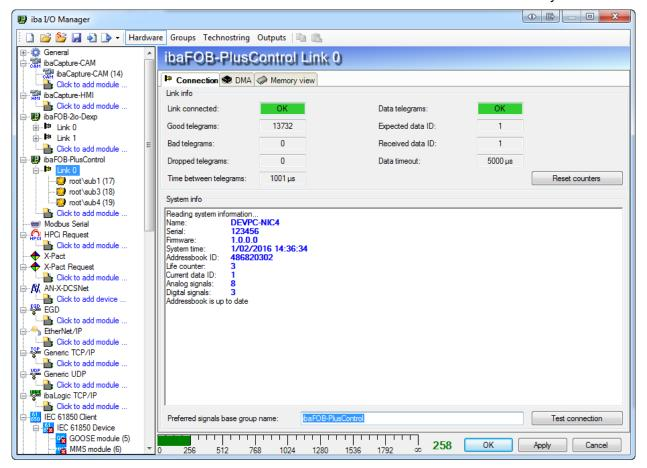
On the link node you can click the "Test connection" button. This will try to communicate with the PlusControl. It will show some information about the connected PlusControl and it will also update the addressbook. The adddressbook contains a list of signals organized in a hierarchical structure. Some signals are marked as preferred signals. IbaPDA will automatically create modules for the preferred signals. There are 3 possibilities when creating the preferred modules:
