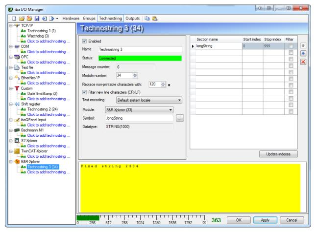
Symbols with data type STRING or WSTRING can be measured as technostring. The B&R-Xplorer technostring uses the connection made by a B&R-Xplorer module to read the string value. This means that the update time of the module is used to read the data. This also means that the actual update time of the module will be influenced by all technostrings linked to the module. The linked B&R-Xplorer module doesn't need to have any analog or digital signals configured.
