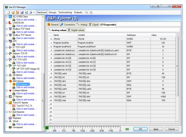
When you have selected all the symbols you want to measure and set the update time then you can apply the configuration. IbaPDA will then make a connection to the PLC and do periodic reads. The module has a fifth tab called *Diagnostics* that shows the values of all the signals that are currently being read from the PLC. The grey rows are signals that are inactive.
