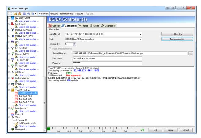
If the symbols are not stored on the PLC, this is the case for bus controllers, then a symbol file needs to be specified. The symbol file is a .tpy file that is generated by the TwinCAT compiler. It is normally located in the same directory as the project file. It is the ibaPDA service that is going to access the symbol file. This means that if the symbol file is located on a network share then you need to specify the UNC path and proper user credentials for it.
