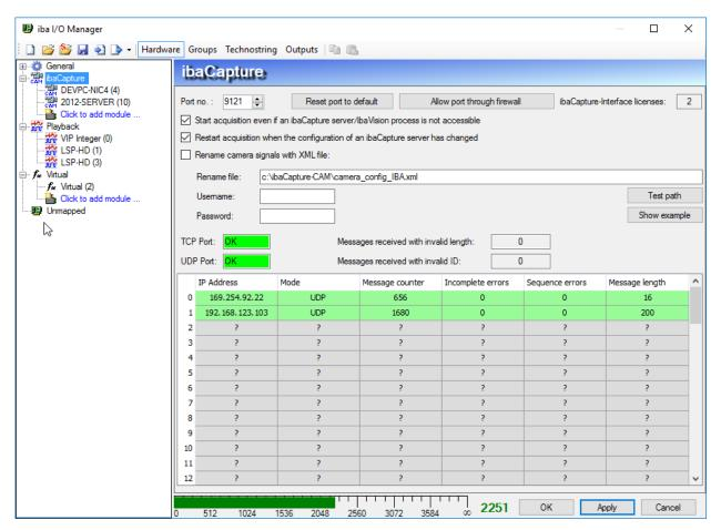
Thirdly ibaPDA can now get a notification from the ibaCapture v4 server that the camera configuration has changed. If ibaPDA detects a change in camera name or a change in index for one of its active cameras then the acquisition can be automatically restarted. You have to enable the option "Restart acquisition when the configuration of an ibaCapture server has changed" on the ibaCapture interface.
