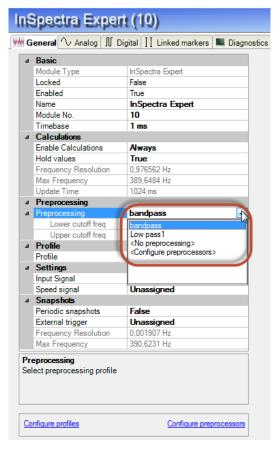
By clicking <Configure preprocessors> in the drop down, you can access the preprocessing manager. In the left part you can create, delete or rename filters which you can reuse in other InSpectra Expert modules.
