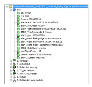
There is a new infofield added to the dat file. It is called start\_event\_type or stop\_event\_type for stop triggers. It determines what type of trigger was used to trigger this dat file. The possible values are:
