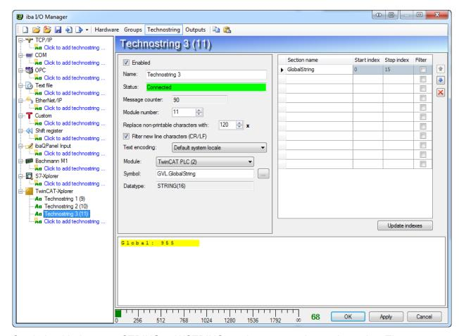
Symbols with data type STRING or WSTRING can be measured as technostring. The TwinCAT-Xplorer technostring uses the connection made by a TwinCAT-Xplorer module to read the string value. This means that the update time of the module is used to read the data. This also means that the response time of the module will be influenced by all technostrings linked to the module. The linked TwinCAT-Xplorer module doesn't need to have any analog or digital signals configured.
