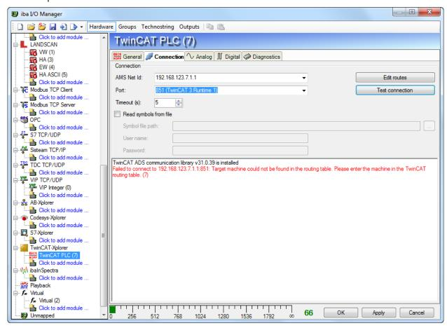
On the connection tab you have to configure the address of the PLC you want to connect to. In ADS the address consists of an AMS Net Id and a port number. The AMS Net Id is the address of an ADS router. It is an extension of the IP address. It consists of 6 bytes. Usually the first 4 bytes are the IP address and the last 2 bytes are 1. The port number determines the ADS device that is connected to the router. There are predefined port numbers for the TwinCAT runtimes:
