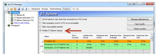
Select the *Outputs* section in the I/O manager. On the general tab of the S7-Xplorer module you can configure the number of analog and digital output signals.
