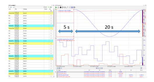
When there is no time span defined in the event configuration then the trend graph will just put the event timestamp in the middle of the X-axis and it won't change the size of the X-axis.
