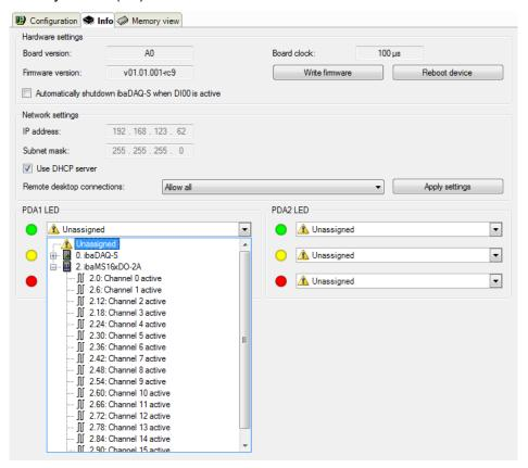
The Info tab shows more specific ibaDAQ-S settings. The hardware board version is displayed as well as the current firmware version. The ibaDAQ-S firmware can be updated here by clicking the Write firmware button and selecting the appropriate iba-file in the dialog that will appear. Note that after a firmware update, the DAQ-S should be powered off and on manually so the FPGA can completely reset.
