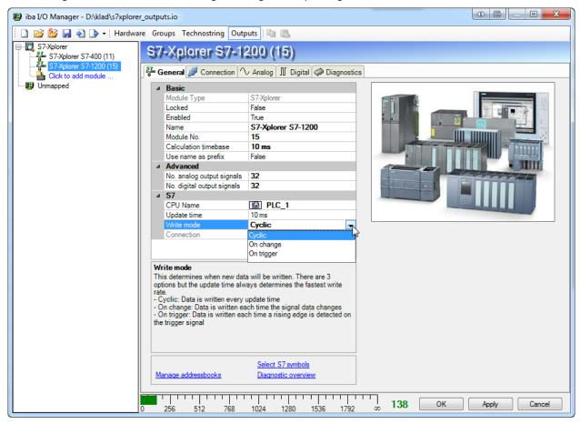
There is a single connection used for both reading and writing data from/to the PLC. So the more you write to the PLC the slower the data will be read. You can determine when data is written to the PLC by setting the *Write mode* property. These are the possible modes:
