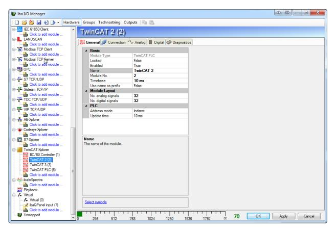
On the general tab of the module you can also configure the update time. This determines how fast ibaPDA tries to retrieve data from the PLC. The actual update time might be higher if the PLC is unable to deliver the data fast enough. You can check the connections table on the TwinCAT-Xplorer interface to see how fast the data is actually coming in.
