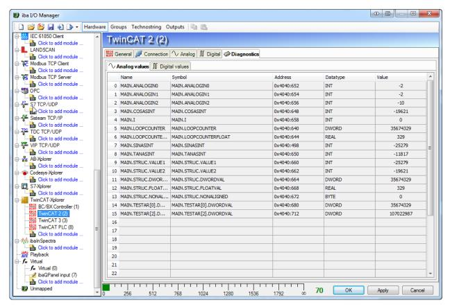
When you have selected all the symbols you want to measure and set the update time then you can apply the configuration. IbaPDA will then make a connection to the PLC and do periodic reads. The module has a fifth tab called *Diagnostics* that shows the values of all the signals that are currently being read from the PLC. The grey rows are signals that are inactive.
