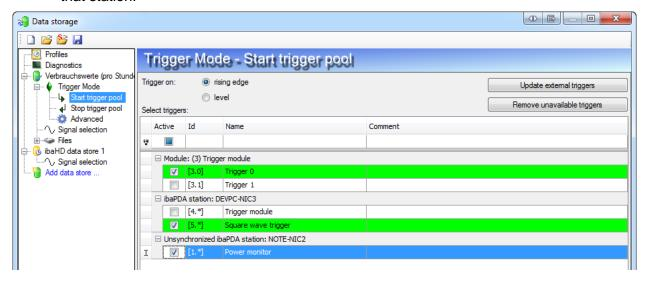
In the trigger pool configuration of a data store you can see the list of available triggers. There are 3 types of triggers:
