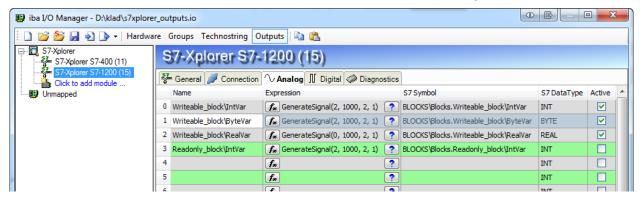
Writing is also supported when using the TCP/IP S7-1x00 connection mode. In this case you have to select the S7 symbols you want to write to.
