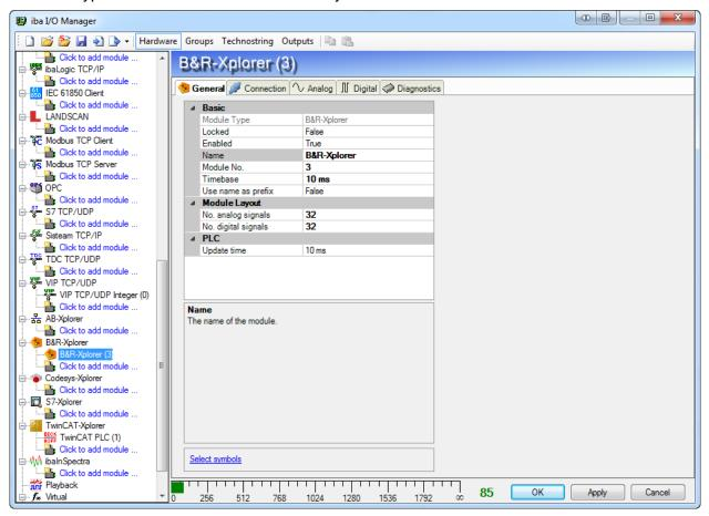
On the general tab of the module you can configure the update time. This determines how fast the PVI manager tries to retrieve data from the PLC. The actual update time might be higher if the PLC is unable to deliver the data fast enough. You can check the connections table on the B&R-Xplorer interface to see how fast the data is actually coming in.
