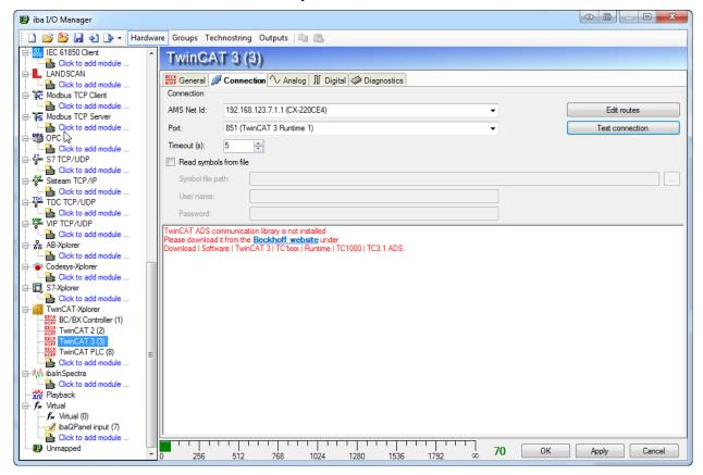
ibaPDA uses the TwinCAT ADS communication library of Beckhoff to connect to the PLCs. This library is not included in the ibaPDA installation. If TwinCAT v2 or v3 is installed on the PC where the ibaPDA service is running then the library will be available. If TwinCAT is not installed
