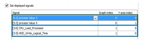
With the example configuration above the commanded trendview is going to display 2 trend graphs. Each graph will show 2 signals from the connected HD Server. Each signal in the first graph will have an own Y-axis and in the second graph they will be using the same Y-axis.
