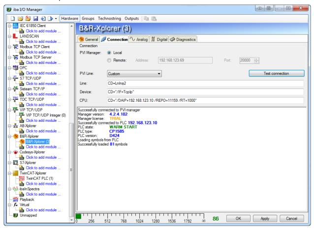
Use the *Test connection* button on the *Connection* tab to try the connection to the PLC. When you test the connection you get some information about the connected PVI manager and PLC. ibaPDA will also load the symbols that are available on the PLC.
