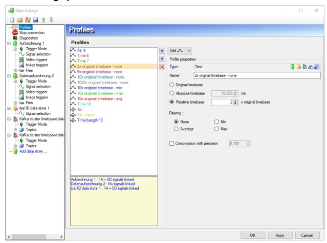
The standard storage profile has been extended with the option to use a relative timebase instead of an absolute timebase. The relative timebase is expressed as a number of times the original timebase.
