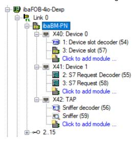
The device slot decoder is the decoder variant of the device slot module. It measures data from a slot of the PROFINET device embedded in the ibaBM-PN. You have to configure the address and data type WORD (little endian) or WORD\_B (big endian) for each decoder.
