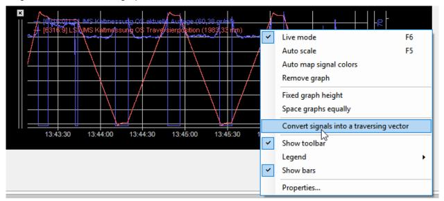
When you have a graph with 2 signals in it then a new command appears in the context menu: Convert signals into a traversing vector. When you click this the traversing vector properties form is opened.
