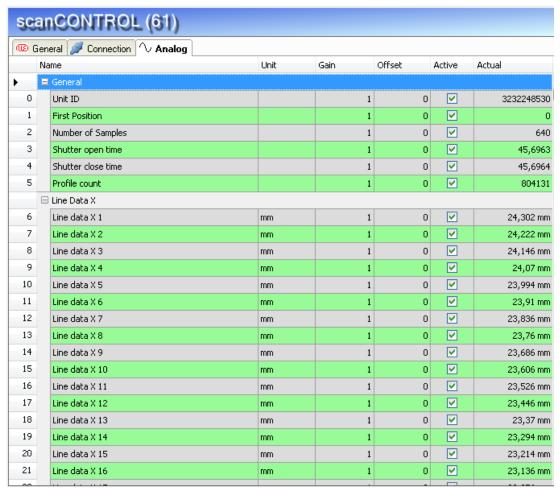
The **Analog** tab of a scanCONTROL module shows the available values. When the acquisition is running, the "Actual" column shows the current value of the available data.
