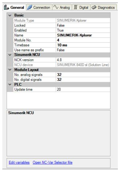
In the General tab of a SINUMERIK-Xplorer module you can configure a couple of settings, apart from the general module settings. The NCK version can be chosen. That version defines which variables can be selected from a tree of documented NCK variables in the Lists Manuals available for that specific firmware version. The NCU device is automatically set when the connection is tested. It is read only and useful for support cases only.
