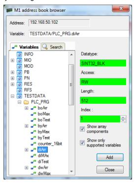
Using the M1 address book browser you can easily add analog or digital signals to the M1-Xplorer module, by double-clicking any variable, or selecting multiple variables and clicking on "Add"
