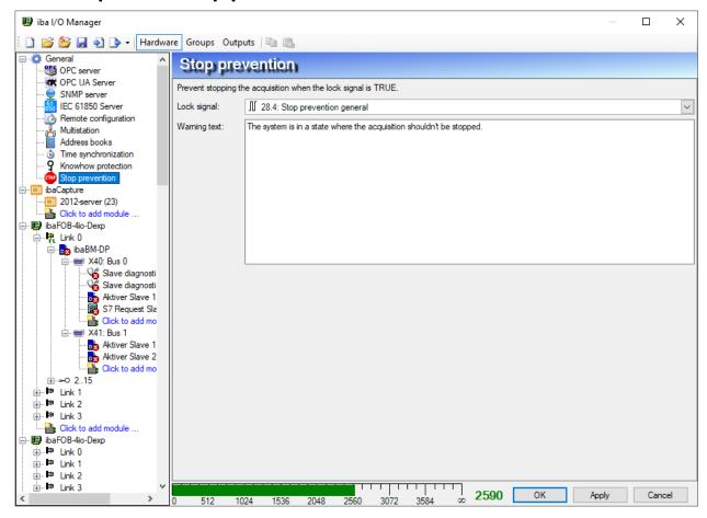
In the I/O manager you can configure a lock signal that signals a situation in which it isn't allowed to stop the acquisition. You can enter your own warning text. This text will be shown in the client when it tries to stop the acquisition while the lock signal is TRUE.
