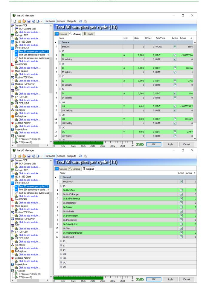
There also exists a custom mode. In this mode you have to configure the sample rate yourself. You can also configure all the signals yourself. You can change the number of signals and you can configure their offsets and data types.
