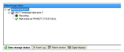
The current status of the DB/Cloud data store can be seen in the *data storage status* window. There are 2 nodes shown per data store. The first one shows the name of the database table and the recording time in brackets. The icon depicts the current state of the recording. There are 3 possible icons:
