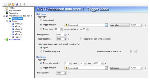
First of all you can select whether you want to write constantly to the database or only triggered. Select *unconditional* as start trigger type when you just want to write all data to the database. In this case all other settings are irrelevant.
