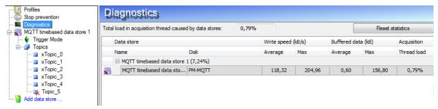
The diagnostics grid in the data storage manager has been extended with the MQTT data store as well. The group shows the load of the writer thread that writes the data to the broker. The disk column shows the address of the database. The write speed shows how fast data is written to the database. The buffered data shows how much data is buffered in ibaPDA. The buffered data will grow when there is no connection to the database. If the size goes over the configured
