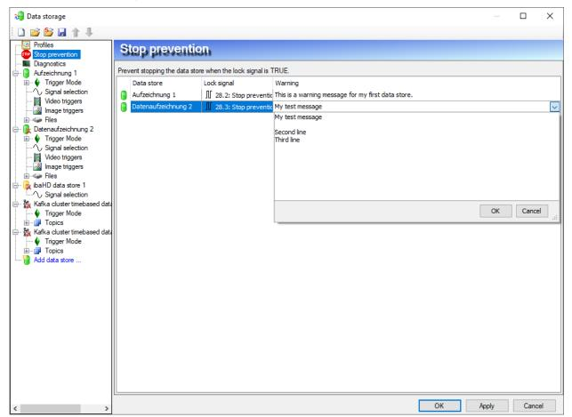
In the data storage manager you can configure a lock signal per data store that signals a situation in which it isn't allowed to interrupt the data store. You can also configure a warning message per store. The message can contain multiple lines.
