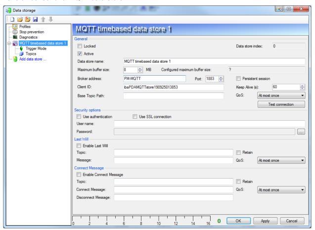
In the MQTT data store you first have to configure to which broker you want to connect. You have to enter the broker address and port number. Also each client connected to the broker must have an unique Client ID. ibaPDA will pre-fill that field. Be careful if you change it,
