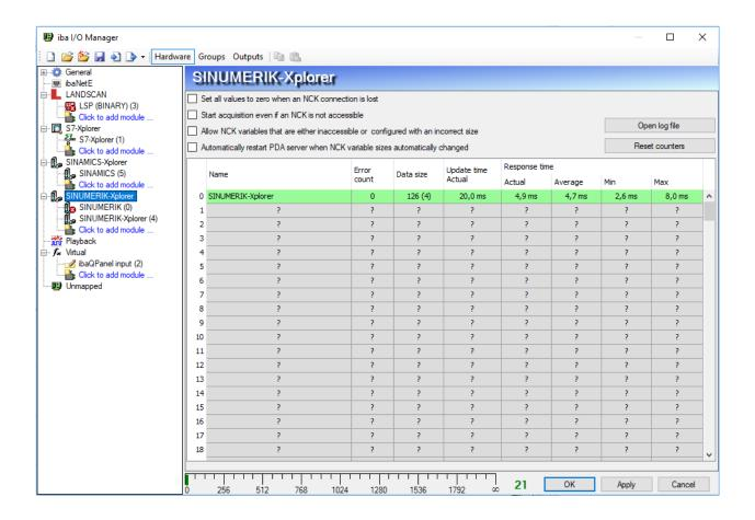
The SINUMERIK-Xplorer interface node contains a table listing all configured and enabled SINUMERIK-Xplorer connections along with some connection status information. The Data size column displays the amount of requested bytes as well as the number of request messages (value displayed between brackets).
