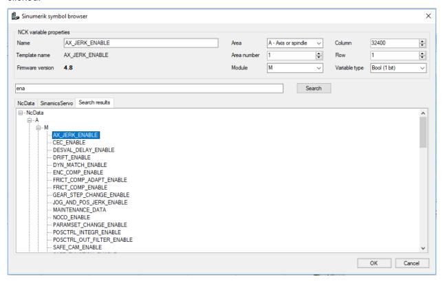
Variables with Bool data type will be digital signals, others will be analog. If you want a digital signal to be shown in the analog tab, you can change its data type to char or byte.
