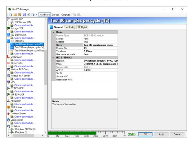
Add an IEC 61850-9-2 module to the IEC 61850-9-2 interface. Each module corresponds with one Sampled Values stream. In the IEC 61850-9-2 section you have to configure all properties of the stream. The first thing to configure is the *Network* property. It determines the network interface where the stream is being received on. The *Mode* determines the format of the Sampled Values and the sample rate. There exist 6 standard modes:
