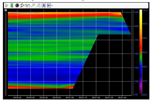
The values between 2 samples of the same zone are interpolated. This means that the data can only be drawn when there are 2 samples available for a zone. That is why you see these sloping edges.
