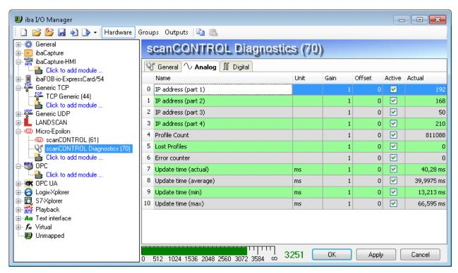
For the Micro-Epsilon devices, a diagnostic module can be configured. It can record the values that are available on the interface table.
