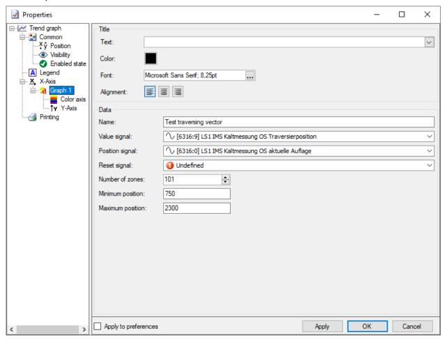
Here you can give the vector a name. You also have to make sure that the correct signals are assigned to the value and position signals. You have to define the number of zones you want to generate. You also need to define the range of the position signal that will be divided into zones. In the example 101 zones will be generated between 750 and 2300. The zones are created as follows. The zone width is calculated as (Max - Min) / (Number of zones - 1). The zones are positioned like this:
