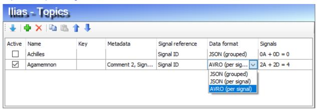
As shown in the picture above, currently encoding data in AVRO is only supported when writing a single record per signal per sample.
