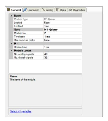
Apart from the standard options that can be found on most other modules, the **Update time** has to be configured. This is the time in ms between two read operations.
