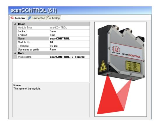
In the General Tab of a scanCONTROL module, apart from the standard options, the profile name can be configured, which is used as name for the automatically generated signal vectors.
