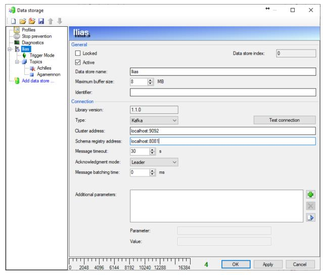
The address and port of the Schema registry can be entered in the main configuration tab of the Kafka data store under **Schema registry address**. When clicking **Test connection** ibaPDA will also try to establish a connection to the Schema registry (if a non-empty address is provided).
