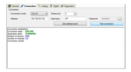
In the **Connection** tab, all parameters to establish a proper connection to the PLC have to be configured:
