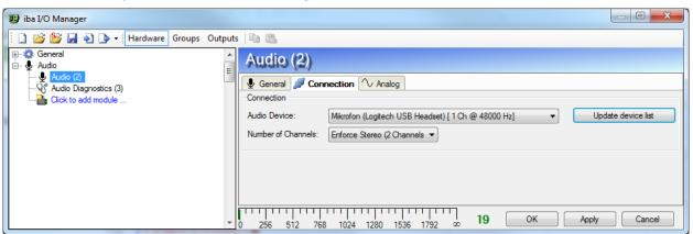
In the **Connection tab**, the desired audio device can be selected from the devices found on the PC hosting the ibaPDA Server. Also the **number of channels** used to record can be changed, the native number of channels can be changed to resample the present channels either to stereo (2 channels) or mono (1 channel).
