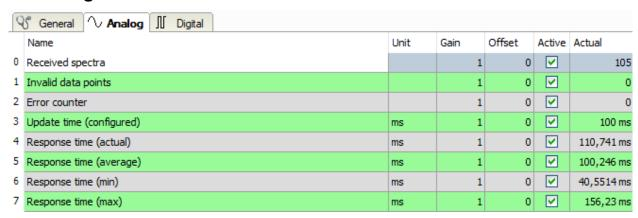
All data displayed in the interface's connection table can also be measured as signals by adding a diagnostics module linked to an FBGS interrogator module. Two extra signals which are not shown in the connection table are available:
