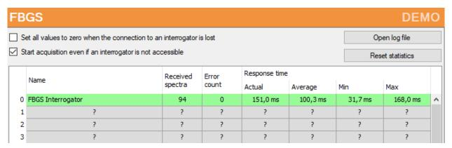
The interface shows a table of all currently configured connections to FBGS interrogators where each connection corresponds to one row in the table. The color of a row has the following meaning:
