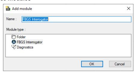
Under the interface node, you can add an FBGS Interrogator module.
