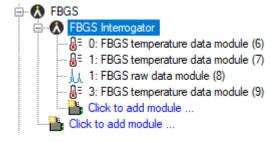
An FBGS Interrogator module by itself does not have any analog or digital signals; these are defined in the interrogator module's submodules or data modules. There are currently two types of FBGS data modules: raw data modules and temperature data modules (these will be explained further on in detail).
