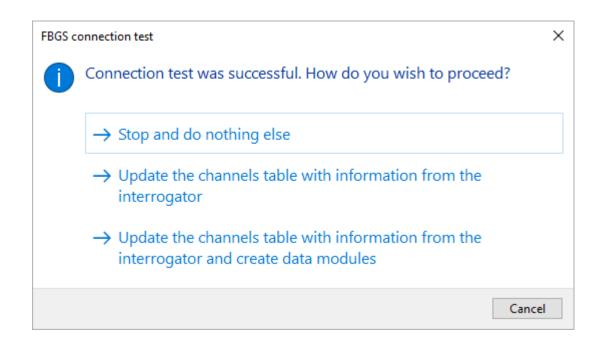
When selecting options 2 or 3, the table in the Channels section will be automatically updated using the information present in the FBGS interrogator. When selecting option 3, ibaPDA will, additionally, create data modules for the active channels.
