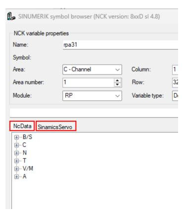
This is no longer the case. NC and SINAMICS servo symbols can be acquired in the same module, as well as symbols of multiple SINAMICS servo drives.
