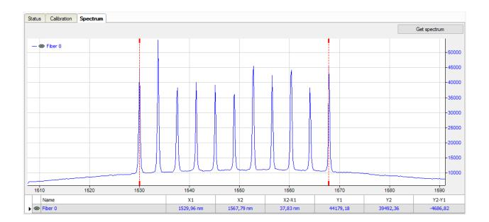
For diagnostic purposes it is possible to retrieve the complete spectrum for each channel by clicking the  $\checkmark$  button. The spectrum will be displayed in the **Spectrum** tab of the lower section of the Connection tab. It is possible to zoom in/out and move the markers (similar to a paused trend graph in ibaPDA). In the Spectrum tab it is also possible to refresh the spectrum using the **Get spectrum** button (which does the same as clicking the  $\checkmark$  button in the toolbar).
