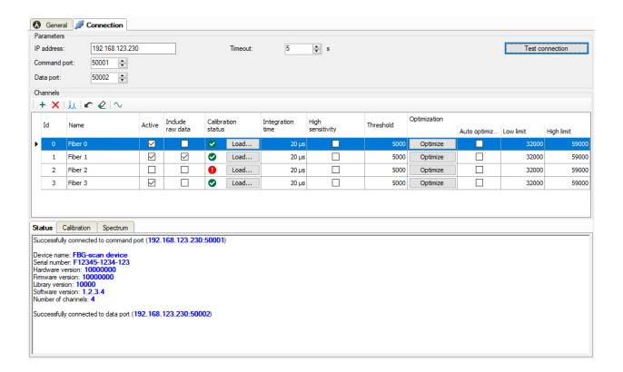
The bulk of the configuration parameters can be found under the **Connection** tab. The Connection tab is divided in three sections: a Parameters section, a Channels section, and a section to display the results of configuration operations.
