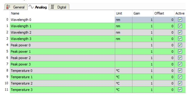
As is the case for the raw data module, the analog signal list is also automatically generated based on the **Channel index** (again to be configured in the data module's **General** tab). The option **Prefix channel index to module name** is available here as well.
