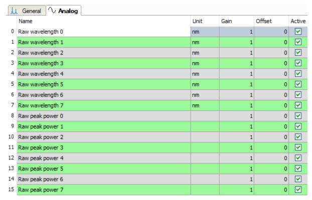
A raw data module simply lists all peak wavelengths and all corresponding peak powers. The analog signal list is automatically generated based on the **Channel index**, which is configured in the data module's **General** tab. In the category **Basic** there is also the option **Prefix channel index to module name**. This makes it easier to distinguish between the data modules of different channels.
