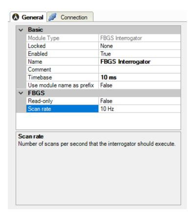
In the **General** tab of an FBGS Interrogator module, the basic module properties can be found alongside some FBGS-specific properties:
