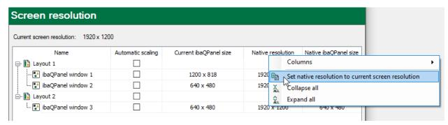
When you open an existing layout with an ibaQPanel window for the first time in the new version, the "Native resolution" is initialized to the current screen resolution and the "Native size" is initialized to the current size.
