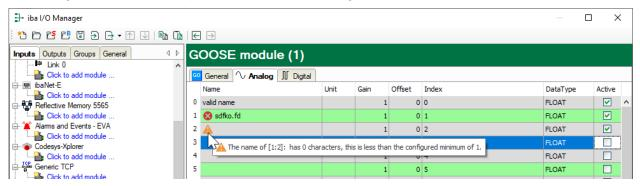
If a signal name does not comply with the rules, then this is indicated in the signal grid via an icon. An error or warning icon will appear and the tooltip will explain which rule is being violated.
