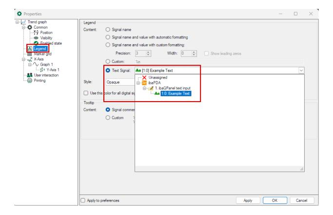
The text signal can contain regular text and legend parameters such as %c1, %x1 etc. (see "Custom" tooltip).
