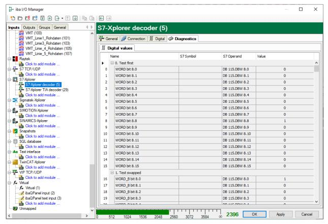
On the Diagnostics tab you can see the measured values of the bits.
