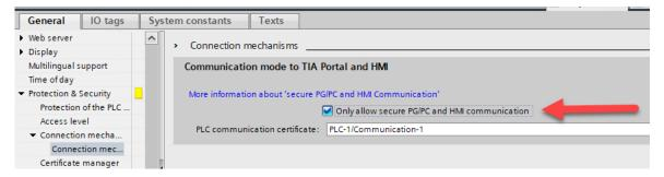
If secure communication is exclusivly configured in the PLC then you have to check the *Use secure communication* checkbox otherwise you will get errors when trying to connect.
