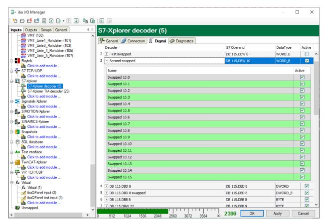
On the *Digital* tab you can configure for each decoder the S7 operand, S7 symbol (if there is an address book configured) and the data type. The data type switches automatically depending on the S7 operand. For 16-bit and 32-bit analog values you can choose between little-endian and big-endian data types. The default is big-endian (WORD\_B and DWORD\_B) because the S7 is big-endian.
