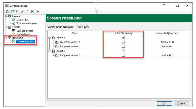
The automatic scaling can be set for every single ibaQPanel or by selecting with SHIFT or CTRL for a group. With CTRL+A all can be selected.
