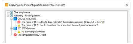
The signal name rules are also checked during the start of the acquisition.
