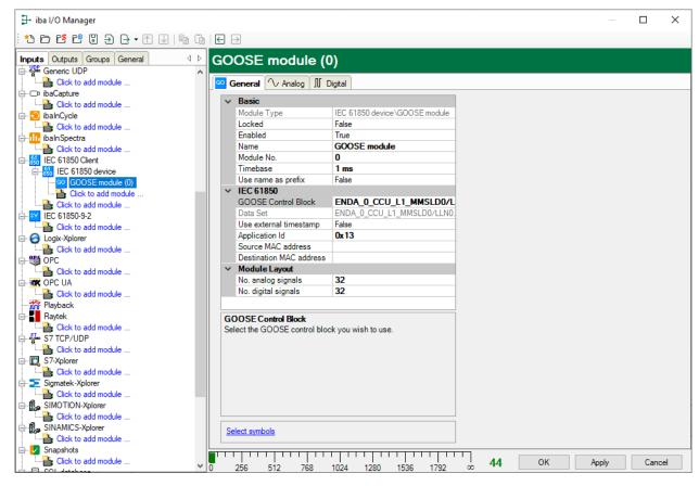
In ibaPDA v8.2.0 you can measure GOOSE messages without an MMS connection to the IED. This means that ibaPDA server doesn't necessarily need to be in the network of the IEDs as long as the GOOSE messages are forwarded to the network ibaPDA server is on. You can configure this via the "Device supports MMS communication" checkbox on the Connection tab of the IEC 61850 device.
