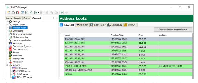
On the *Address books* node on the *General* tab you can now also see the IEC 61850 address books. In the *Modules* column you can see the modules that use a particular address book. You can double-click on it to jump to that module. The *Delete selected address books* button can be used to delete address books. IbaPDA server v8.2.0 is required for deleting address books.
