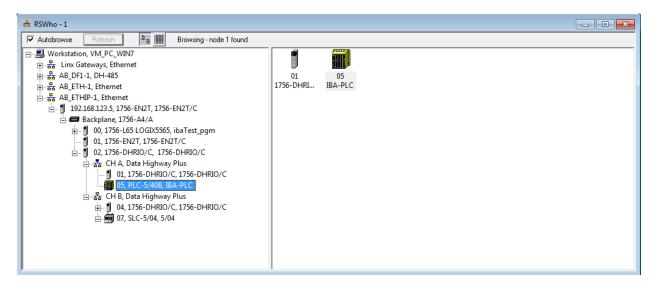
In the screenshot you see that the ControlLogix at IP address 192.168.123.5 has a 1756-DHRIO card in slot 2. This card has 2 DH+ channels. On channel A a PLC-5/40B with DH+ address 5 is connected. On channel B an SLC-5/04 with DH+ address 7 is connected.
