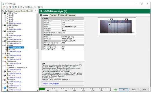
The SLC-5/04 from the example can be reached via *Path Backplane*, 2, *B*, 07. *Backplane*, 2 brings us again to the 1756-DHRIO. *B*, 07 goes to octal address 7 on channel B, which is the SLC-5/04.
