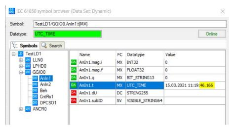
*ibaPDA* does not internally support a *Timestamp* data type. In order to still be able to measure time information, e.g. for checking the latency period and the jitter of IEC 61850 data, the seconds and milliseconds fraction is acquired from a *Timestamp* as a float value.
