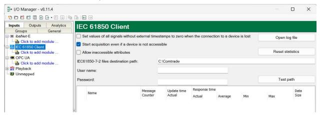
The modules for which the connections exist are identified by name in the first column (left) grouped by IEC 61850 devices.
