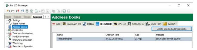
The *Modules* column displays the modules that use a specific address book. You can double-click on it to jump to this module.
