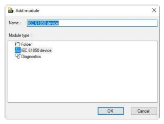
Add a module by clicking below the interface. Select the module type "IEC 61850 device" and click on <OK>.
