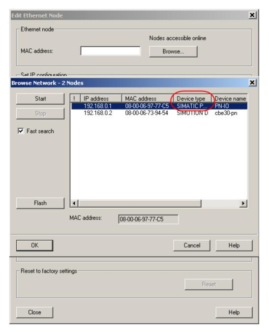
Beneath set IP-configuration (1) must a suitable address for the system be put in. In our example is the address 10.105.51.124 and subnetmask 255.255.0 used.
