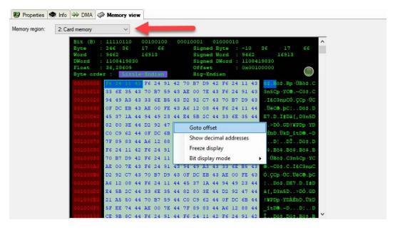
Usually there is no need to access this dialog. The blinking green light indicates a running system in which the visualization is refreshed. The offset addresses equal the address entries in the signal tables of the data modules only when the *Card memory* is selected as indicated by the red arrow above.
