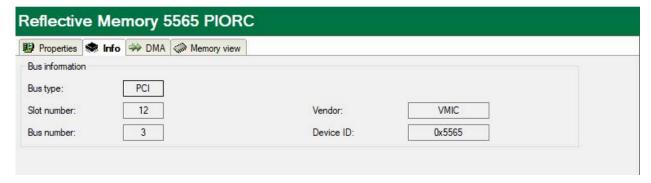
Besides vendor name and device ID you'll find the bus type, slot and bus number. If the fields are empty or contain implausible values, then the board is plugged into a wrong PCI slot.
