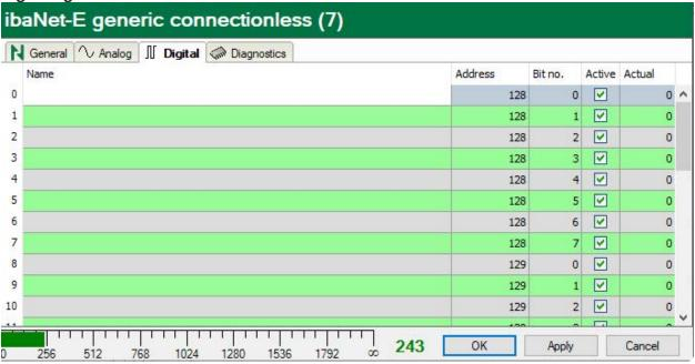
You can assign name and address to the digital signals. Moreover, you can enable or disable the signals.
