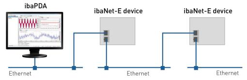
Connection via a switch or router:
