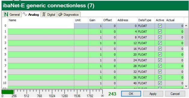
You can assign name, unit, scale factor, address and data type to the analog signals. Moreover, you can enable or disable the signals.
